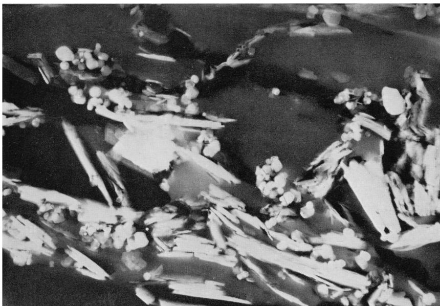
Fig. 14 —Good titanium dioxide efficiency: ultra-thin cross-section of paper with clay and titanium dioxide [ \times 13\ 250 ]
