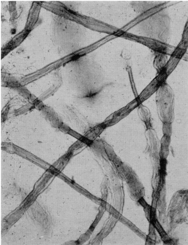
Fig. V —Kraft pulp refined in PFI mill at 20 per cent consistency for 4 000 rev: fibres treated with cupriethylenediamine [ \times 100 ]
