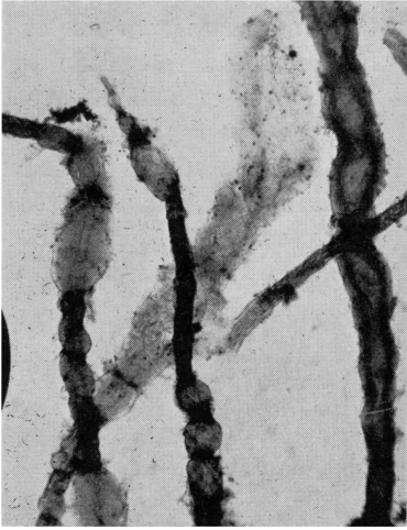
Fig. T —Kraft pulp refined in PFI mill at 5 per cent consistency for 4 000 rev: fibres treated with cupriethylenediamine [ \times 100 ]
