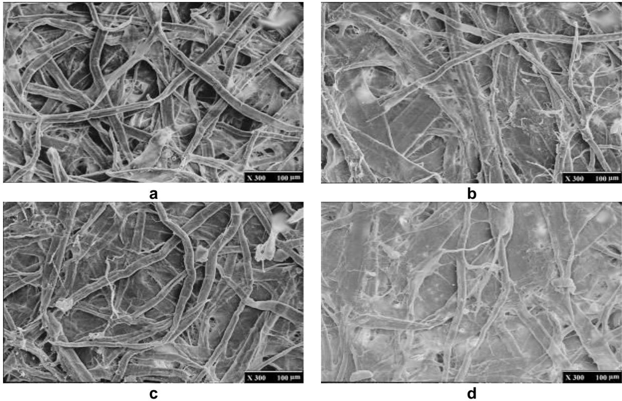
**Fig. 3.** The surfaces of paper made from chemical pulp and a) 0% nano-cellulose, b) 0.3% nano-cellulose, c) 0.6% nano-cellulose, and d) 0.9% nano-cellulose
