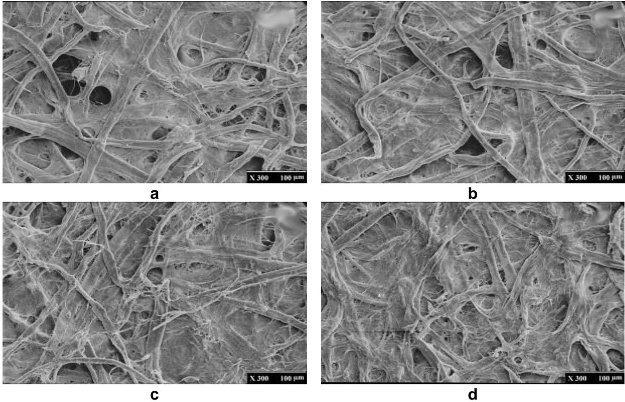
**Fig. 5.** The surfaces of papers made from 15% chemical pulp and 85% cotton pulp and a) 0% nano-cellulose, b) 0.3% nano-cellulose, c) 0.6% nano-cellulose, and d) 0.9% nano-cellulose
