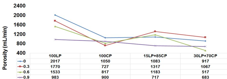
**Fig. 1.** The effect of nano-cellulose and pulp and paper type on porosity
