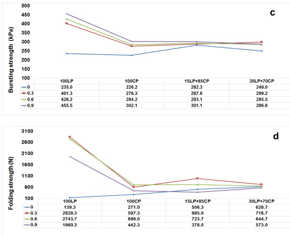
**Fig. 2.** The effect of nano-cellulose and pulp and paper type on a) Tensile strength, b) Tearing strength, c) Bursting strength, and d) Folding strength
