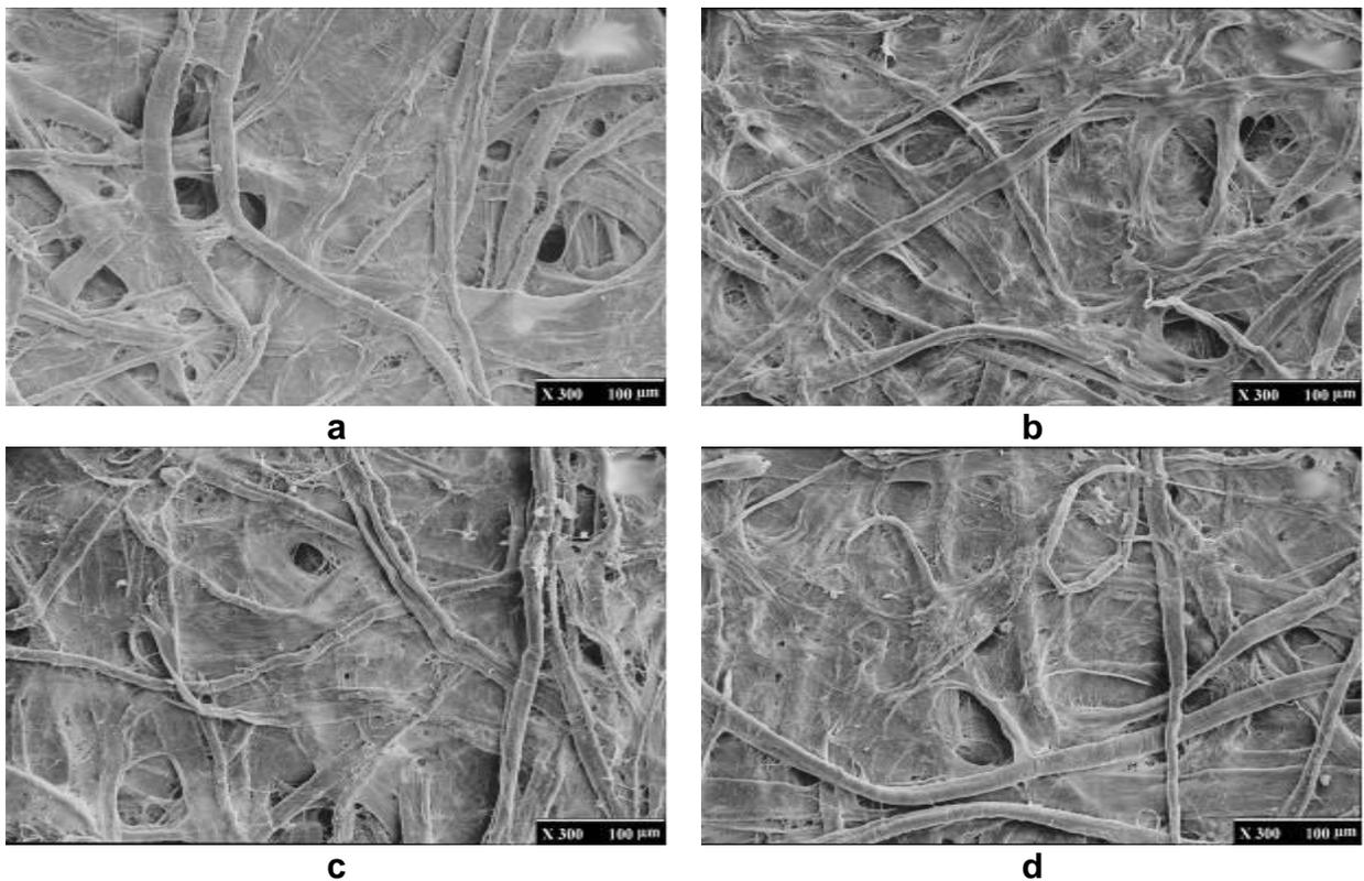
**Fig. 6.** The surfaces of papers made from 30% chemical pulp and 70% cotton pulp and a) 0% nano-cellulose, b) 0.3% nano-cellulose, c) 0.6% nano-cellulose, and d) 0.9% nano-cellulose
