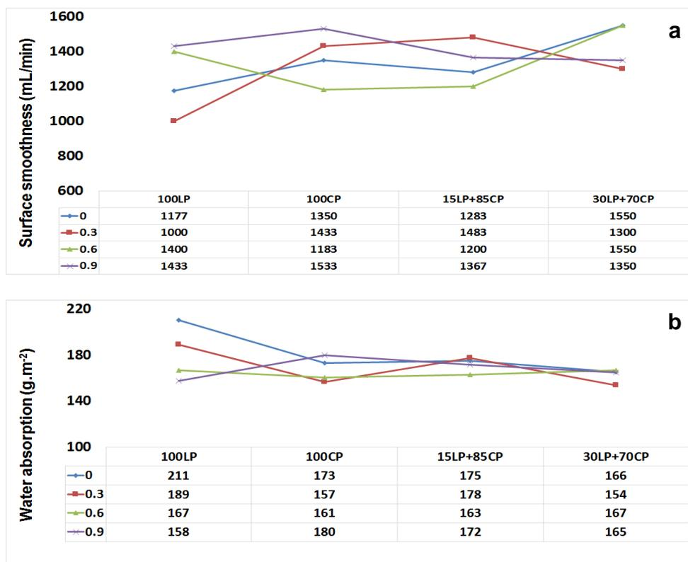
**Fig. 7.** The effect of nano-cellulose and pulp and paper type on a) Surface smoothness, and b) Water absorption
