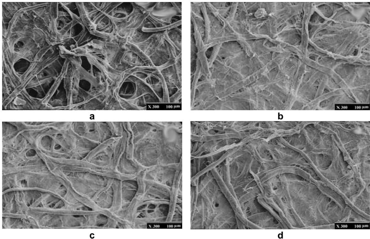
**Fig. 4.** The surfaces of paper made from cotton pulp and a) 0% nano-cellulose, b) 0.3% nano-cellulose, c) 0.6% nano-cellulose, and d) 0.9% nano-cellulose
