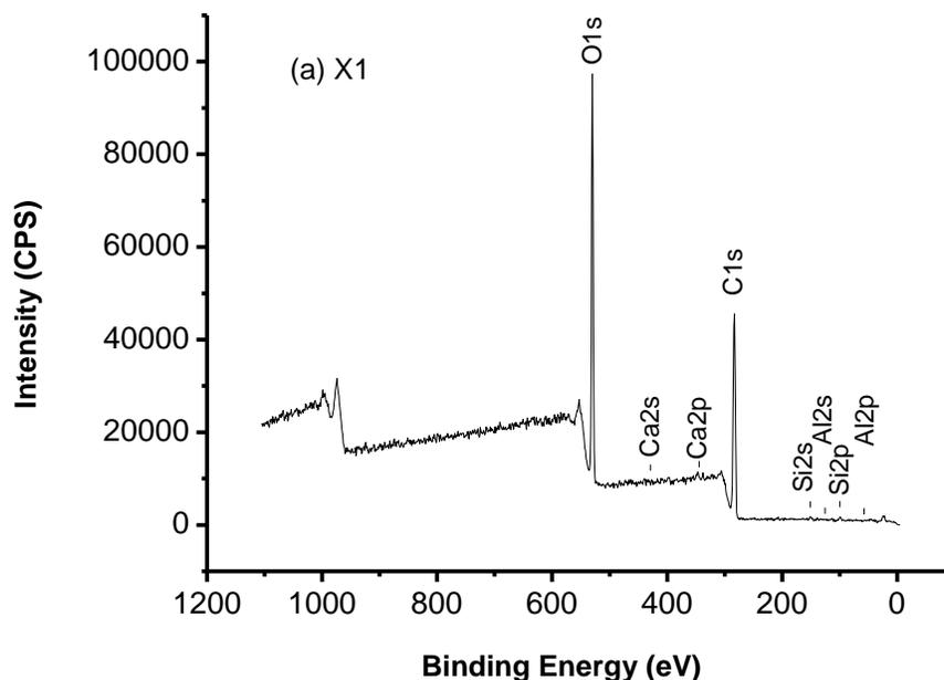
**Fig.1a.** Survey XPS spectra from the surface of laccase/mediator-treated unbleached pulp
