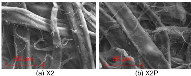
**Fig. 7.** SEM Images of the Lipase-treated unbleached and bleached pulps at 1000x magnification
