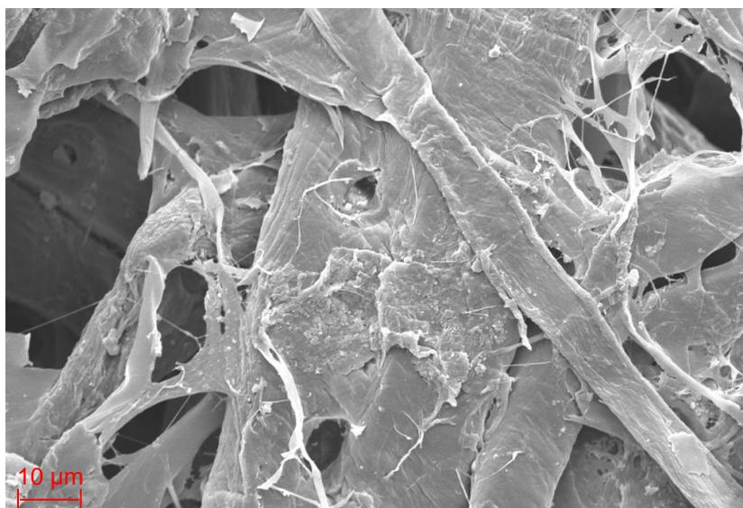
**Fig. 5.** SEM Image of the unbleached pulp at 1000x magnification
