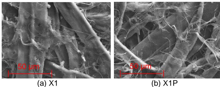
**Fig. 6.** SEM Images of the laccase/mediator-treated unbleached and bleached pulps at 1000x magnification
