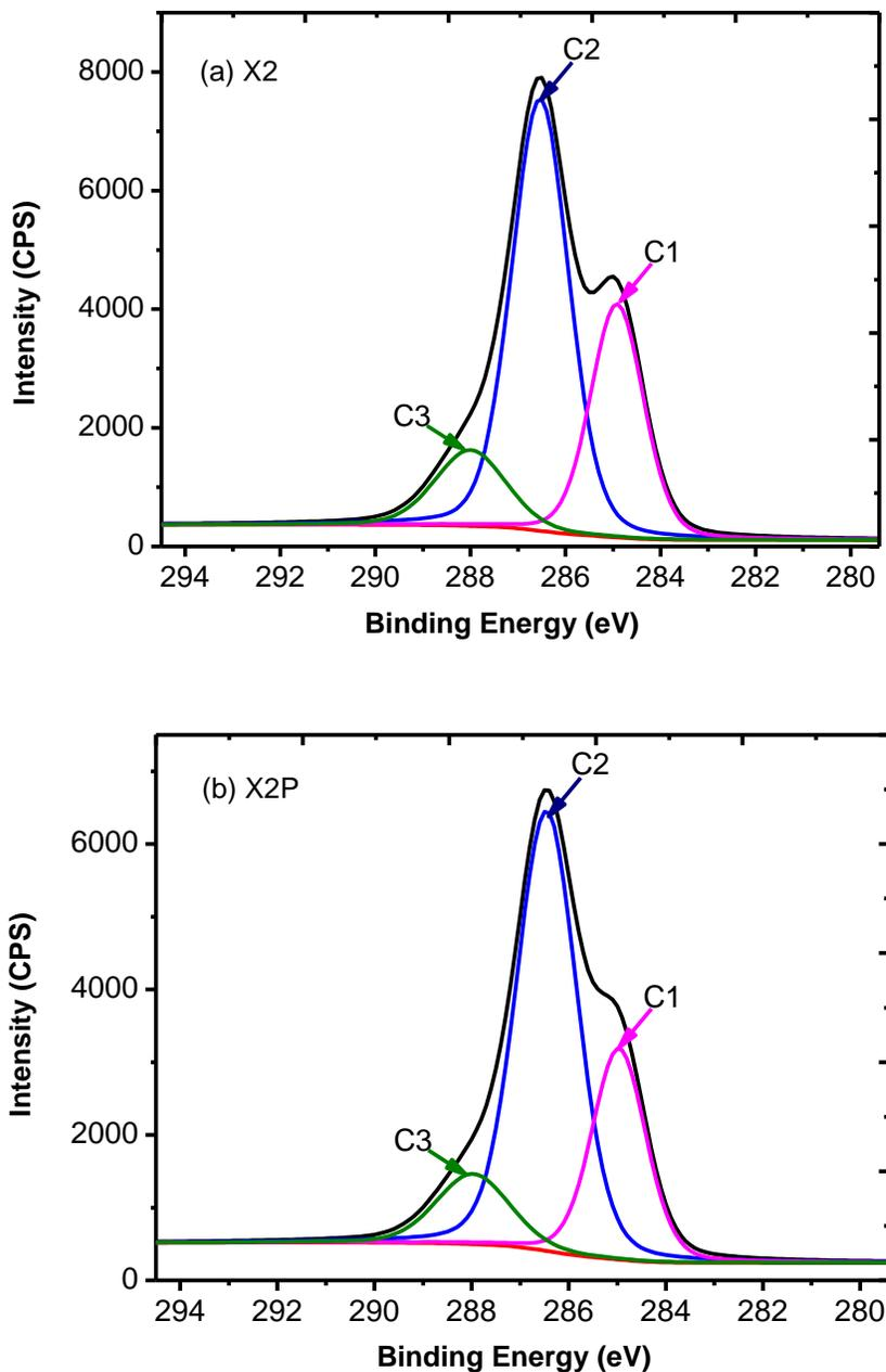
**Fig. 4.** High-resolution XPS C1s spectra from the surface of lipase-treated unbleached pulp (a) and bleached pulps (b)
