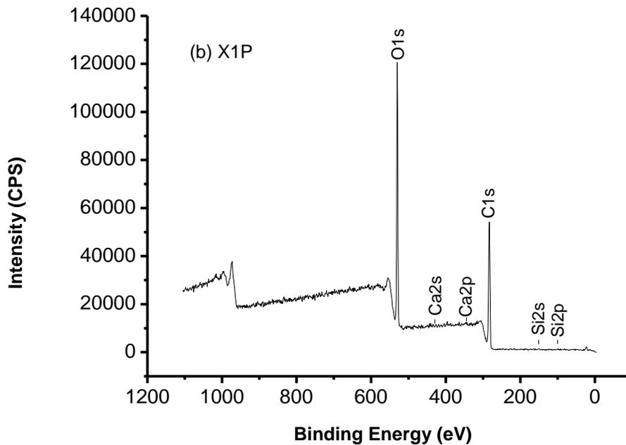
Fig.1b. Survey XPS spectra from the surface of laccase/mediator-treated bleached pulp
