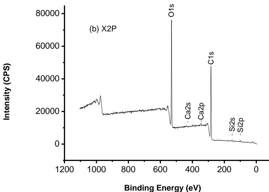
**Fig. 2b.** Survey XPS spectra from the surface of lipase-treated bleached pulp
