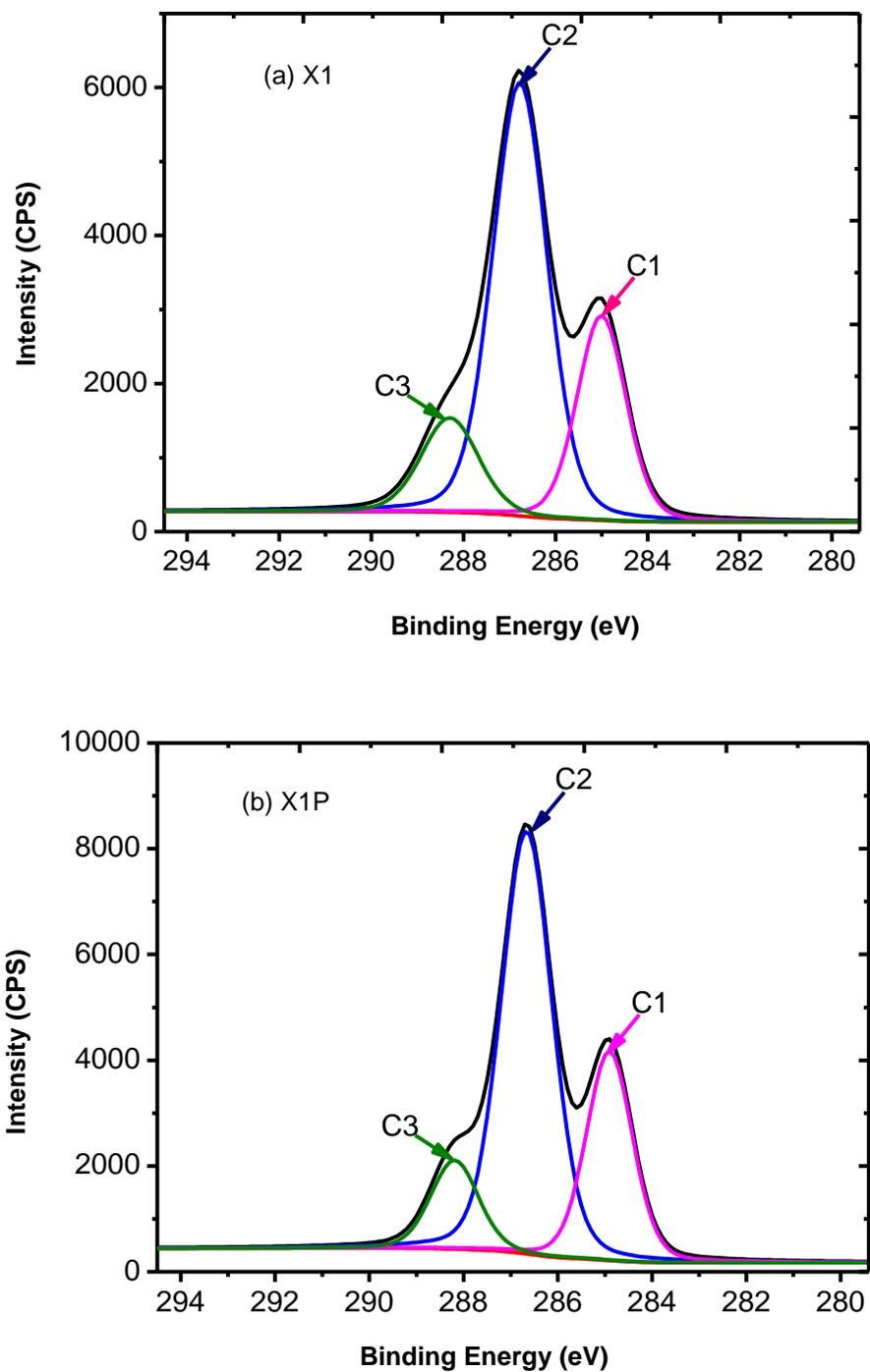
**Fig. 3.** High-resolution XPS C1s spectra from the surface of laccase/mediator-treated unbleached pulp (a) and bleached pulps (b)
