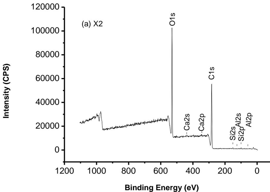
Fig. 2a. Survey XPS spectra from the surface of lipase-treated unbleached pulp
