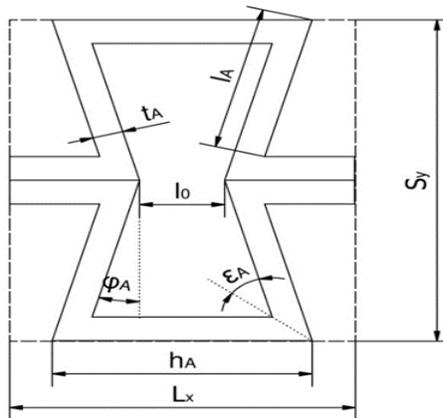
**Fig. 1.** Elementary core cell, where:  $t_A$  (mm): thickness of cell wall;  $l_A, h_A$  (mm): length of cell wall side,  $\varphi_A, \epsilon_A$  (°): interior angles of a cell;  $S_y, L_x$  (mm): overall dimensions of cell;  $l_0$  (mm): distance between cell walls
