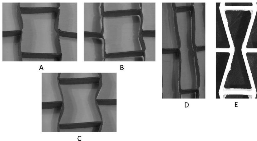
**Fig. 8.** Images of elementary cells in cores: A through D: paper cores; E: WoodEpoxy® core
