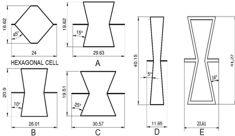
**Fig. 2.** Elementary core cells: Hexagonal cell, the reference cell with relative density  $\rho_A = 0.0249$ ; A through D: paper cells; E: WoodEpoxy® cell
