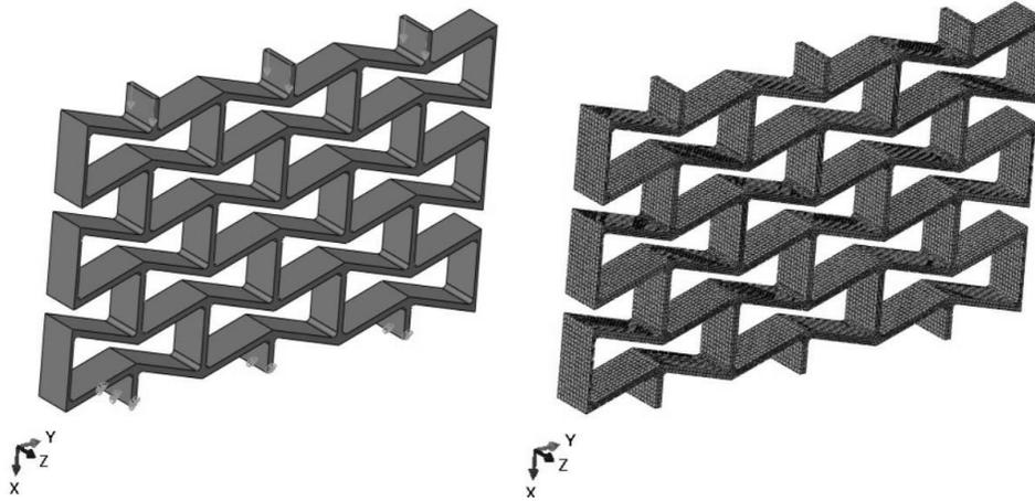
**Fig. 3.** An example model of a core used in numerical computations; Left is a diagram of loads, and right is a mesh grid for the model
