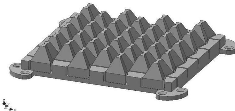
**Fig. 4.** An example mold to manufacture the selected paper core
