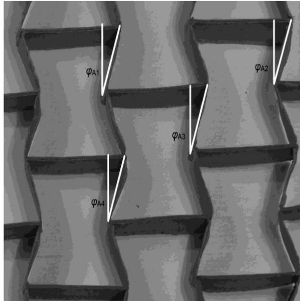
**Fig. 9.** Different angles of inclination of tested core D fragment
