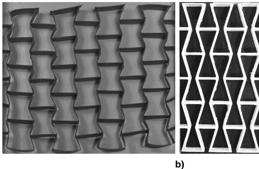
**Fig. 5.** a) Example paper core type D, b) core E manufactured from WoodEpo<sup>x</sup>®
