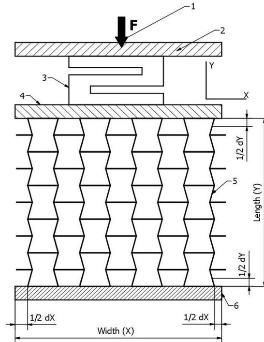
**Fig. 6.** The testing stand: 1) pressing screw, 2) sensor platten, 3) ZEMIC H3-C3-25kg-3B sensor, 4) sample platten, 5) tested sample, and 6) support
