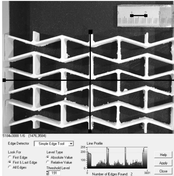
**Fig. 7.** The method to measure strain: detection of gauge points
