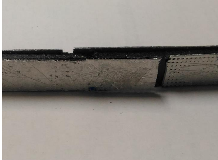
Fig. 3. Failed pristine FF specimen from the fatigue test
