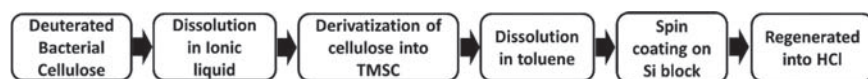
Figure 1. Synthesis process of deuterated cellulose film spin coated from deuterated cellulose bacteria.
