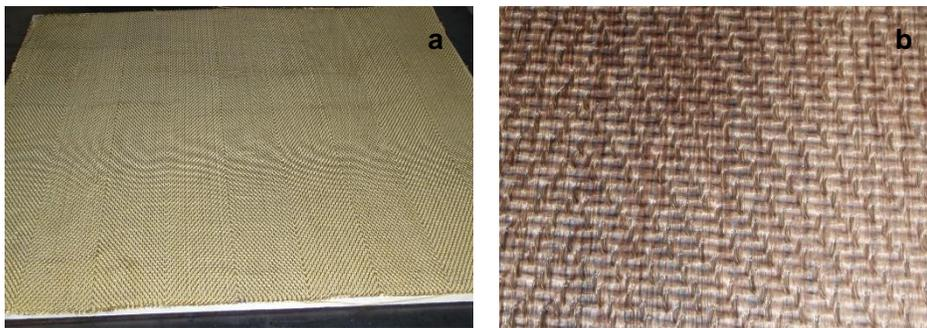
**Fig. 4.** Both sides of red oak specimens were covered with copper wire mesh before densification (a), and the specimens' surface became rough after densification (b)
