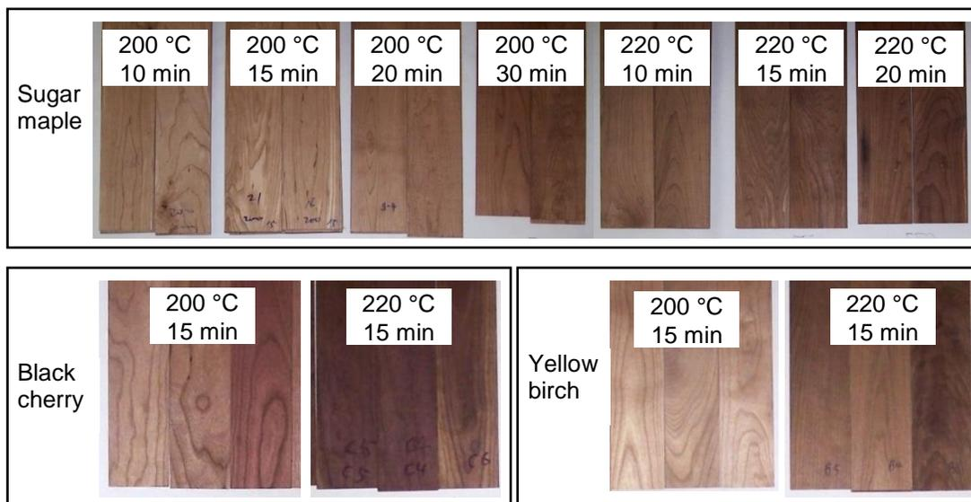
**Fig. 8.** Specimens after densification with SMMLs at different temperatures with different durations
