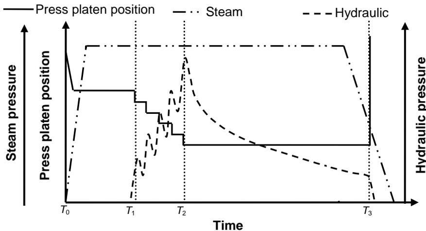
**Fig. 2.** Schematic diagram of the densification process: pre-treatment ( $T_0$  to  $T_1$ ), compression ( $T_1$  to  $T_2$ ), and post-treatment ( $T_2$  to  $T_3$ )
