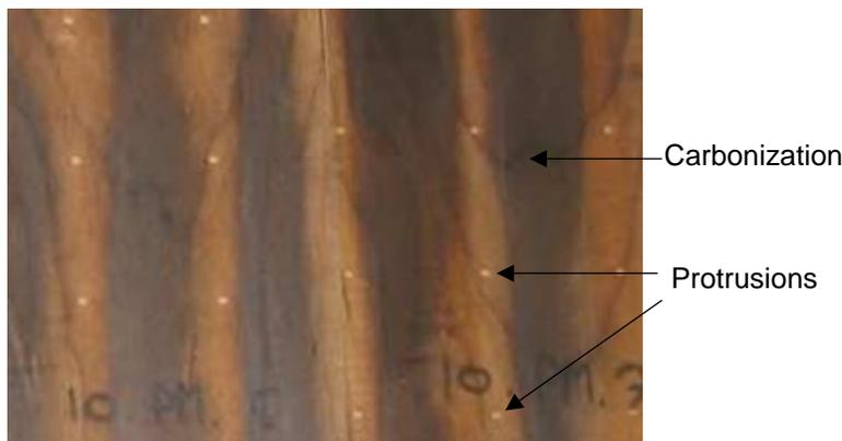
**Fig. 7.** Protrusions and carbonization on specimens after the previous THM densification treatment
