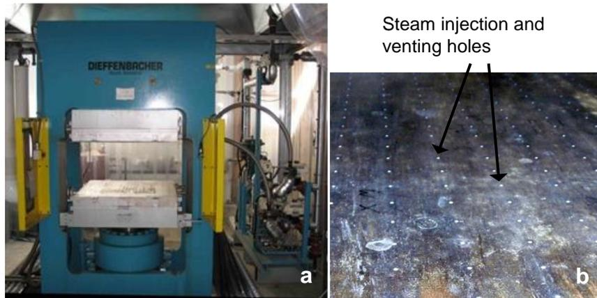
**Fig. 1.** Steam injection hot press used for the densification treatment: (a) 862 mm × 862 mm hot press, (b) steam injection and venting holes on both the upper and lower platens
