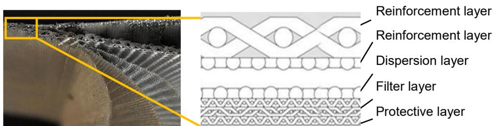
**Fig. 6.** Five-layer SMML used to cover wood specimens
