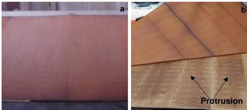
**Fig. 3.** Both sides of the sugar maple specimens were covered with steam-permeable and heat-resistant fabric before densification (a), and protrusions surrounded with dark color were found after densification (b)
