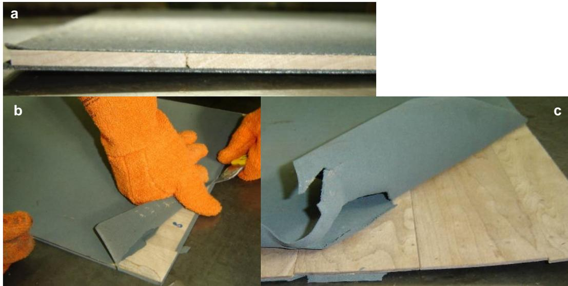
**Fig. 5.** Both sides of specimens were covered with open-celled metal foams with interconnected pores (a), specimens' surface became very rough and the metal foams stuck to wood after densification (b and c)
