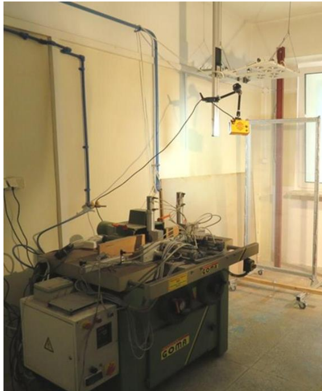
Fig. 2. General view of the test stand - woodworking machine with accessories and the tested shield
