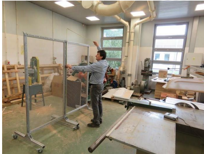
Fig. 10. A woodworking shop worker demonstrates, based on his personal experience, a suitable height in his opinion for shields protecting against kickback from a circular sawing machine; two shields were placed next to each other to increase the width of the separated zone
