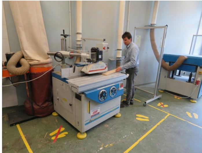
Fig. 9. A shield separates two workstations, which limited the kickback hazard zone and reduced the risk of the operator being knocked down by another worker
