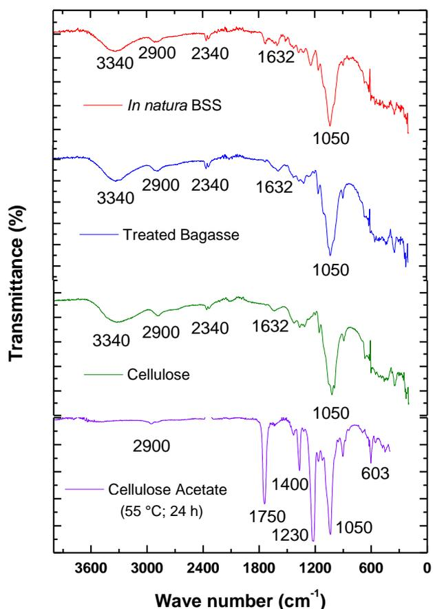
**Fig. 7.** FTIR spectra of the *in natura* BSS, treated bagasse, cellulose, and cellulose acetate
