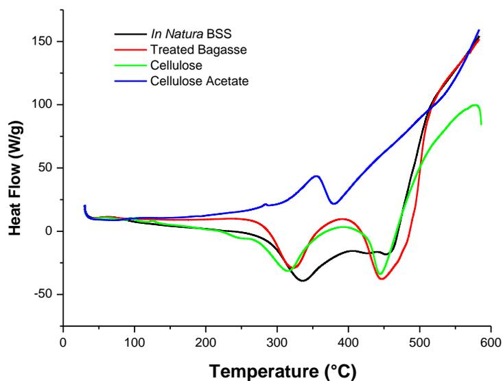
**Fig. 9.** DSC curves of the *in natura* BSS, treated bagasse, cellulose, and cellulose acetate
