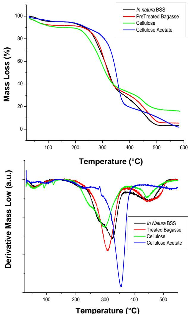
**Fig. 8.** TG (a) and DTG (b) of the *in natura* BSS, treated bagasse, cellulose, and cellulose acetate
