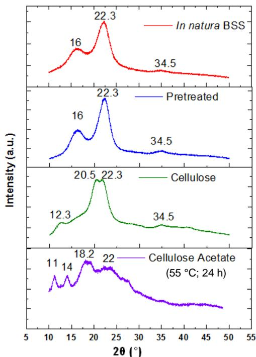
**Fig. 6.** XRD patterns of the *in natura* BSS, treated bagasse, cellulose, and cellulose acetate
