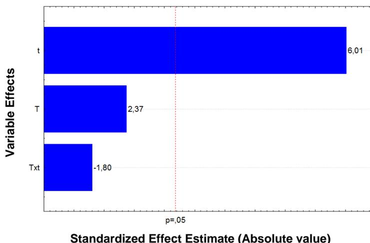
**Fig. 4.** Pareto chart for the cellulose acetate DS from the BSS where  $t$  represents time,  $T$  temperature and  $Tx t$  the interaction between temperature and time.
