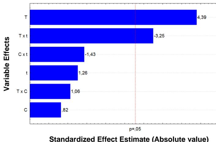
**Fig. 2.** Pareto chart of the variable effects on the percentage of lignin removal in the pretreatment of the BSS with alkaline hydrogen peroxide
