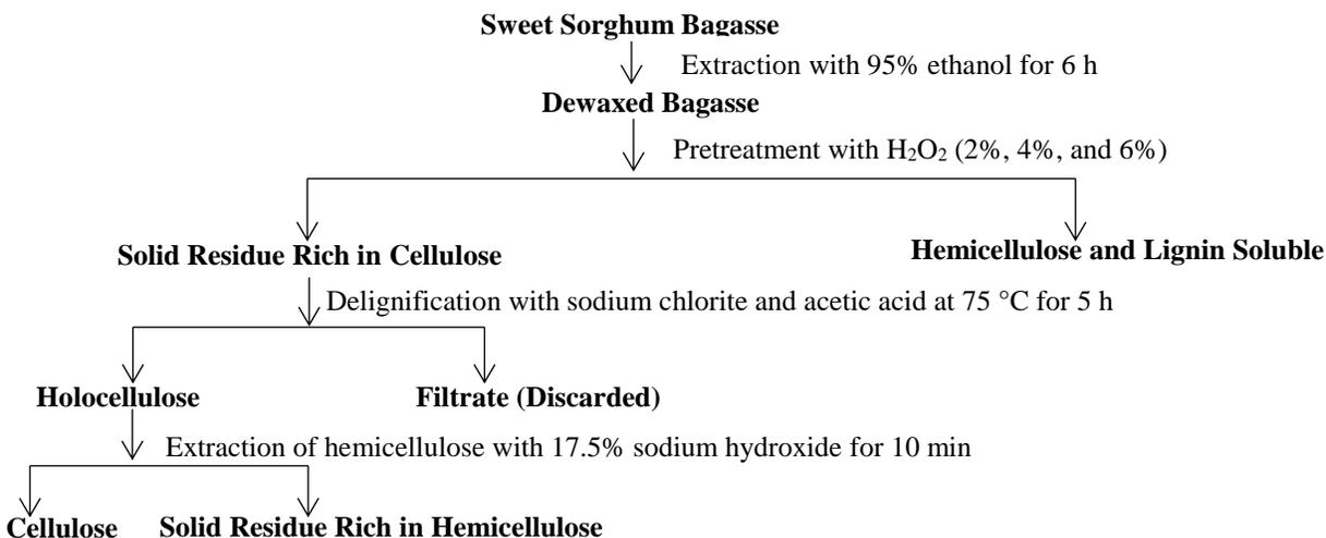
Fig. 1. Representative scheme of cellulose isolation
