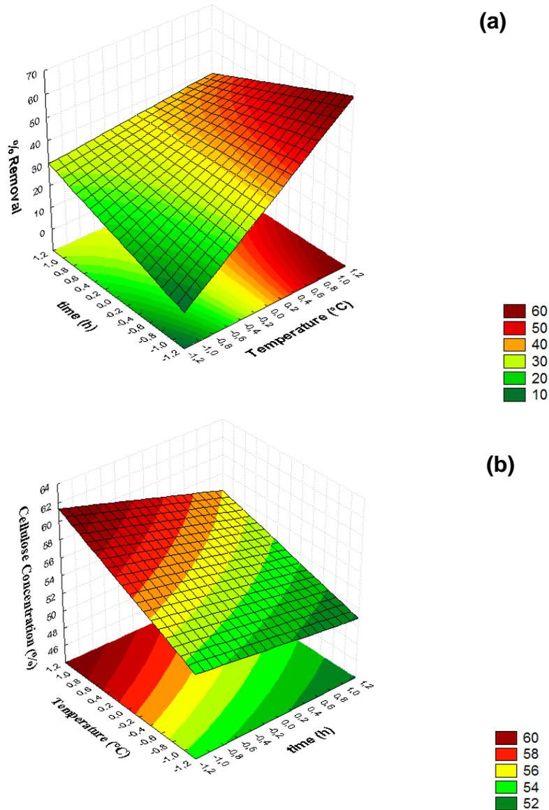
**Fig. 3.** Response surface for the lignin removal percentage (a) and cellulose concentration percentage (b) as a function of the temperature and time, with the concentration held at the +1 level (6%)
