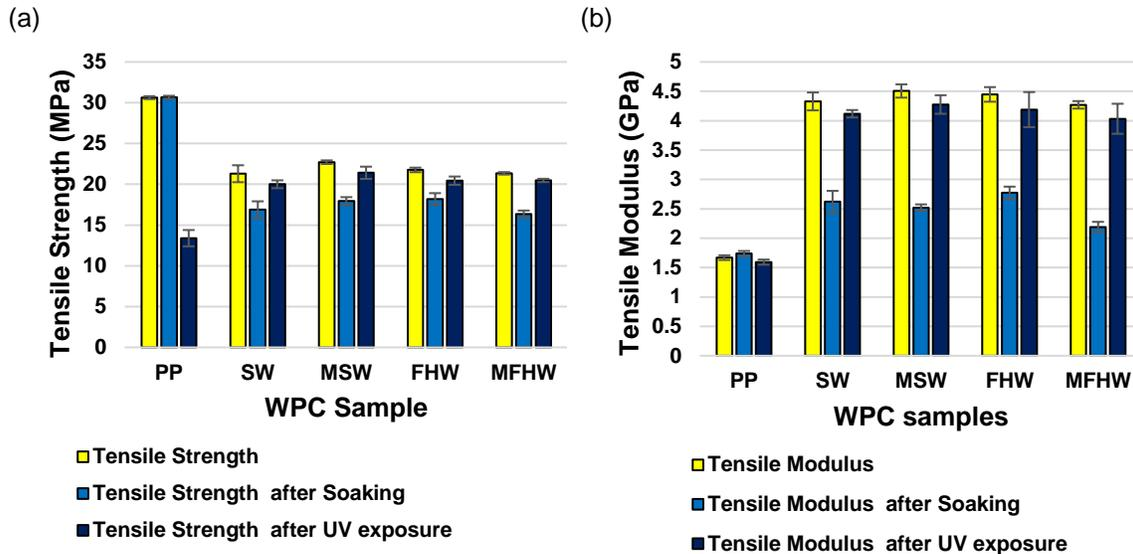
**Fig. 1.** Tensile Properties of the WPC samples before and after soaking in water and exposure to UV; SW – birch sapwood; MSW – modified birch sapwood; FHW – false heartwood; and MFHW – modified false heartwood
