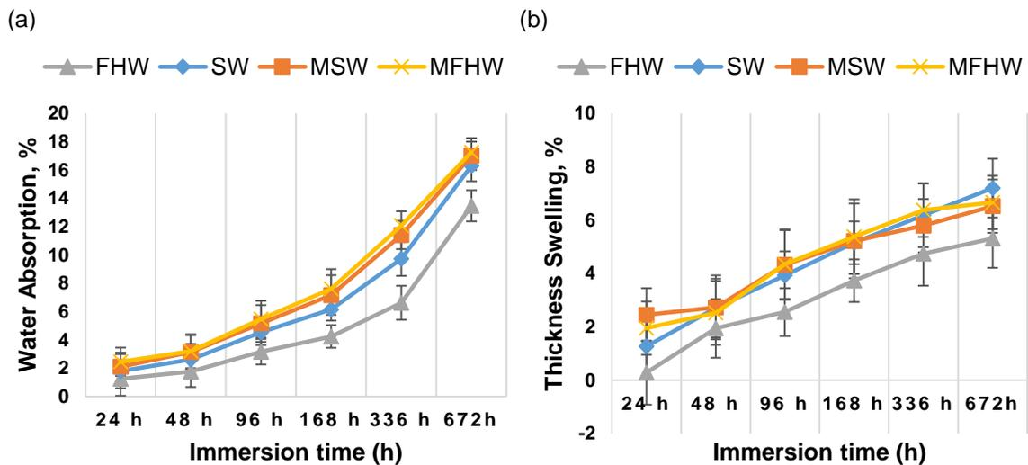
**Fig. 3.** Water absorption and thickness swelling of the WPC samples: SW – birch sapwood; MSW – modified birch sapwood; FHW – false heartwood; and MFHW – modified false heartwood
