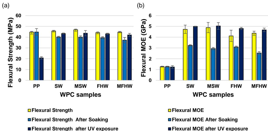
**Fig. 2.** Flexural Properties of the WPC samples before and after soaking in water and exposure to UV; SW – birch sapwood; MSW – modified birch sapwood; FHW – false heartwood; and MFHW – modified false heartwood
