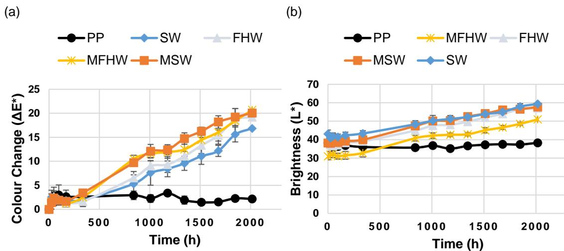
**Fig. 4.** Colour and brightness change of the WPC samples: SW – birch sapwood; MSW – modified birch sapwood; FHW – false heartwood; and MFHW – modified false heartwood
