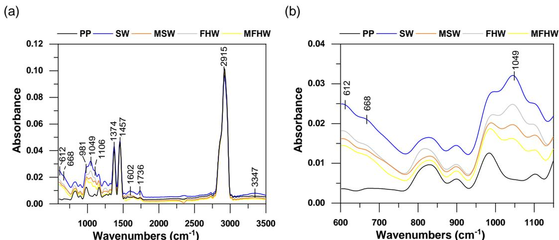
**Fig. 5.** FTIR spectra of the composites and neat PP: SW – birch sapwood; MSW – modified birch sapwood; FHW – false heartwood; and MFHW – modified false heartwood
