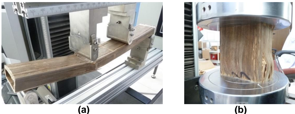
Fig. 3. Test destruction examples of MPB. (a) Bending failure; (b) Compression failure
