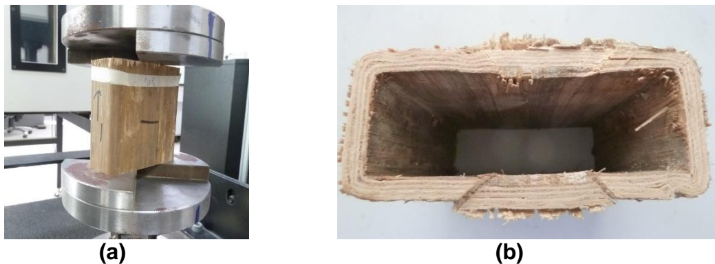
Fig. 4. Shear test destruction of MPB. Shear properties (a) test schematic and (b) specimens
