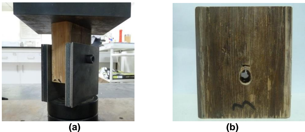
Fig. 6. (a) Double shear single bolt connection and (b) failure schematic
