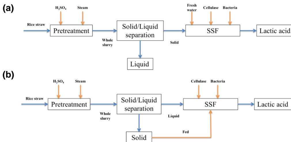
**Fig. 1.** Proposed lactic acid production processes: (a) conventional SSF with the addition of fresh water; and (b) integrated SSF with whole slurry
