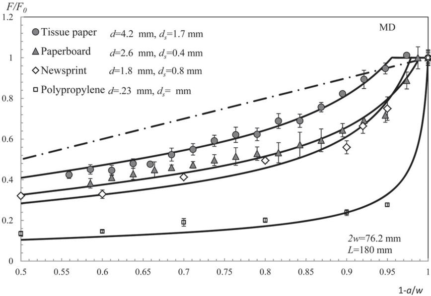
**Figure 19.** DENT results of load ratio versus relative ligament length for various papers in MD direction. Solid lines represent Equation (6). Dash-dot line represents notch-insensitive response  $F/F_0=1-a/w$ .
