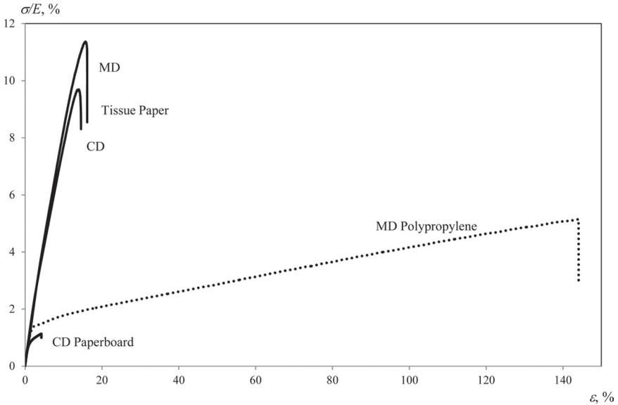
**Figure 15.** Stress-strain curves for tissue paper and polypropylene film. Stress is normalized to Elastic modulus.
