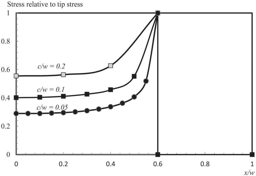
Figure 6. Stress distribution along ligament for three characteristic lattice sizes with  $a/w=0.4$ .
