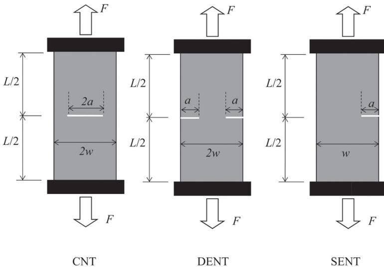
**Figure 1.** Typical geometries for in-plane fracture tests with paper.
