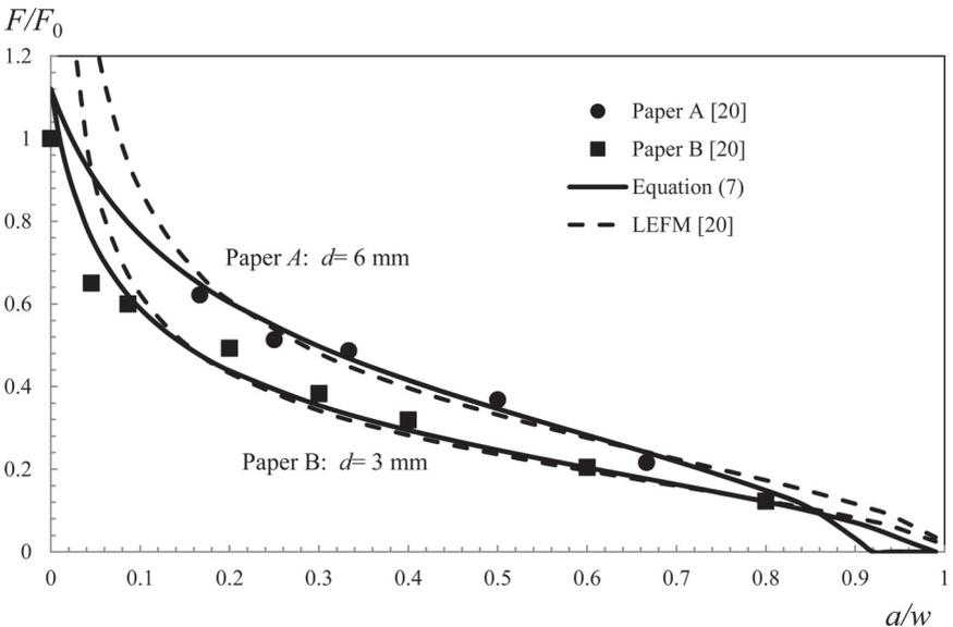
Figure 10. Comparison of Equation (6) to LEFM using CNT data from [20].
