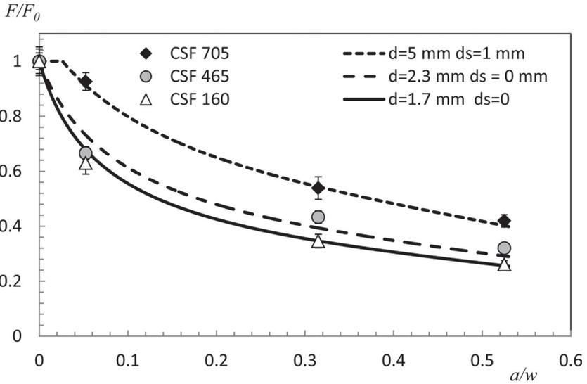
Figure 21. Effect of beating on DENT fracture sensitivity for handsheets, 50 g/m<sup>2</sup>.
