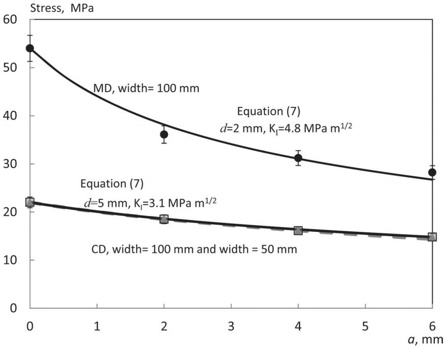
Figure 7. DENT fracture tests of a copy paper [6] compared to Equation (7).
