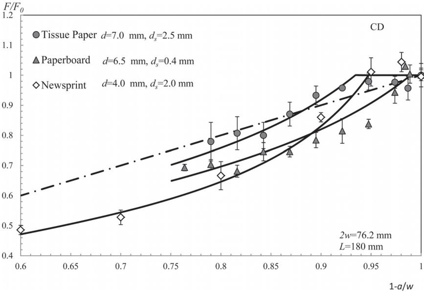
**Figure 20.** DENT results of load ratio versus relative ligament length for various papers in CD direction. Solid lines represent Equation (6). Dash-dot line represents notch-insensitive response  $F/F_0=1-a/w$ .
