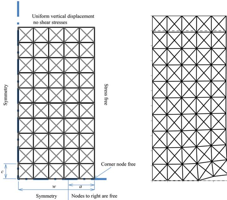
**Figure 3.** Flawed lattice model (1/4 of DENT specimen). (Right: deformed lattice)
