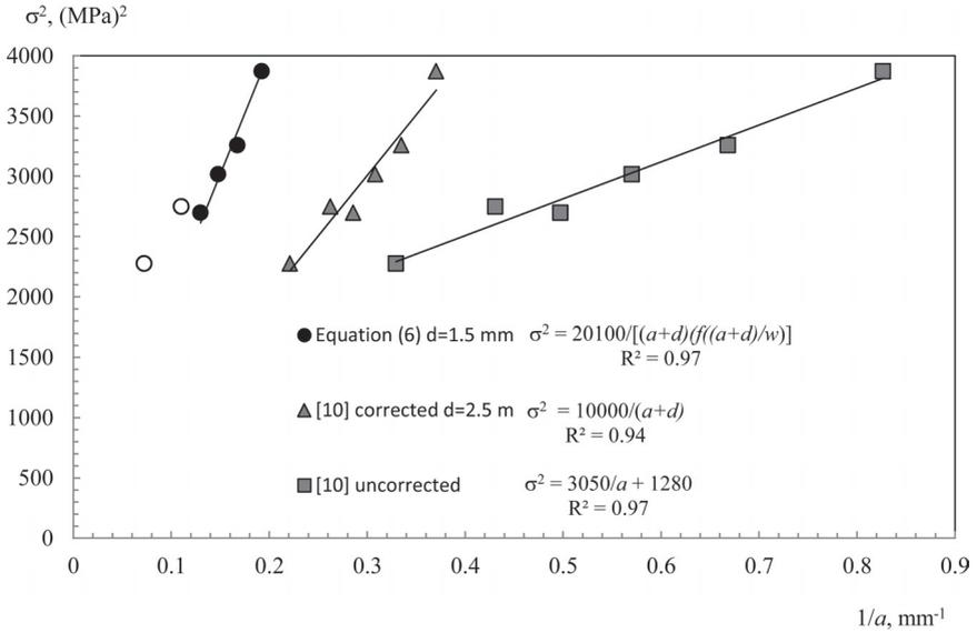
**Figure 8.** Fracture results from Fig 4 of Ref. [10] and Equation (6) with  $d=2.5 \text{ mm}$ .
