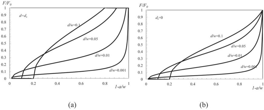
**Figure 2.** Fracture load ratio as a function of ligament length for various characteristic fracture lengths for DENT. (a) All structural  $d=d_s$ , (b) all material  $d_s=0$ .
