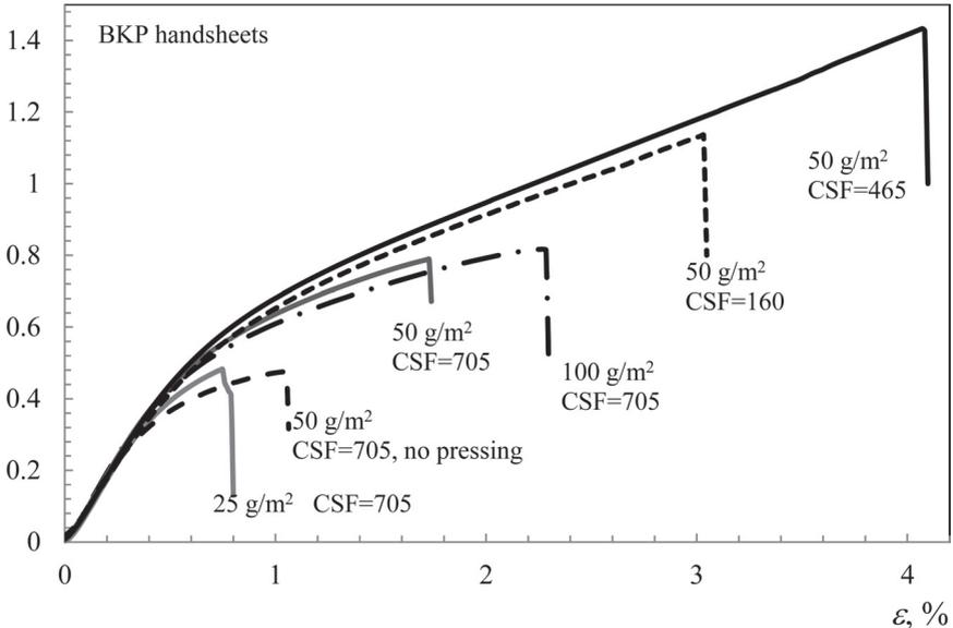
Figure 16. Stress-strain curves for handsheets.
