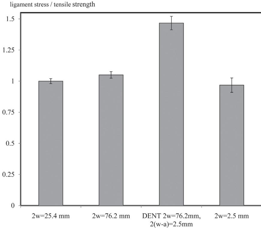
**Figure 26.** Comparison of tensile strength versus deep-notched DENT strength for MD copy paper.
