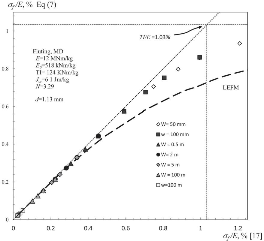
**Figure 12.** Comparison of Equation (6) with that from Reference [17] for MD Fluting.
