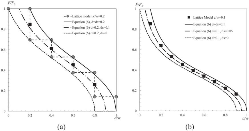
**Figure 4.** Load ratio versus crack length for flawed lattice model. Black squares represent the average load ratio that occurs before and after the release of a node at a crack length of  $a$ . (a) is for a lattice with  $w=5c$  and  $L=50c$ , and (b) is for  $w=10c$  and  $L=100c$ .
