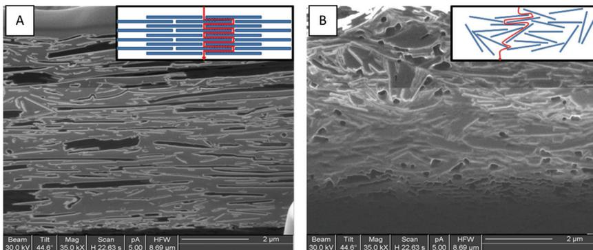
**Figure 4.** Focused ion beam images showing the alignment of the kaolin particle filled latex barrier layer. A: Highly aligned high shape factor kaolin. B: Poorly aligned low shape factor kaolin. The tortuosity of the structures is shown schematically in the inserted images [35].
