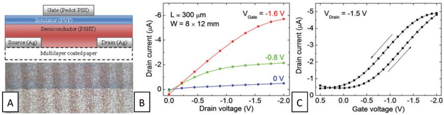
**Figure 13.** A: Schematic and optical image of a roll-to-roll printed HIFET. Output (B) and transfer (C) characteristics of the transistor on the multilayer curtain coated paper. Reproduced with permission. Copyright 2012, Elsevier [29].
