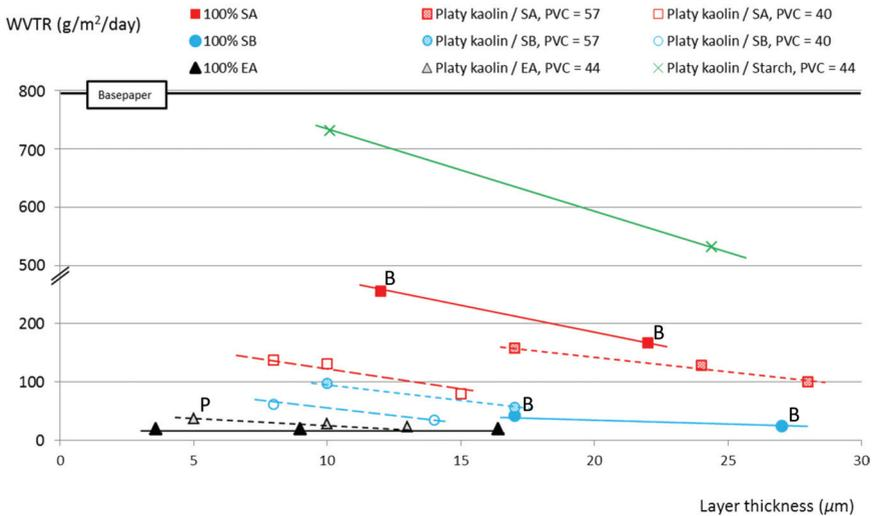
**Figure 5.** Barrier properties against water vapor (WVTR) at 23°C and 85% RH as a function of barrier layer thickness. The values are average values of three parallel measurements, with a negligible standard deviation. (B = Tendency for blocking, P = risk for pinholes). Note the discontinuous Y-axis scale.
