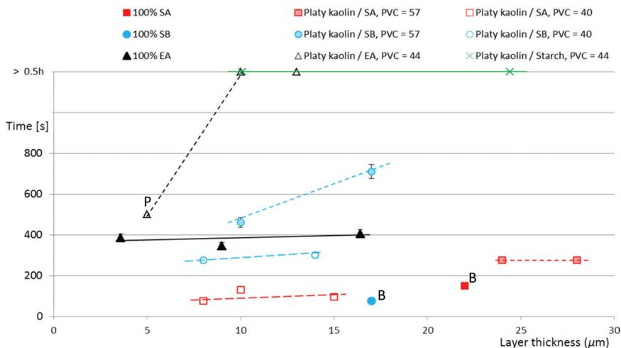
**Figure 6.** Barrier properties against ortho-dichlorobenzene. The figure shows the time in seconds for the liquid to penetrate the substrate. (B = Tendency for blocking, P = risk for pinholes). Penetration time measured with prism method presented in Figure 2B [50].
