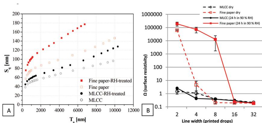
**Figure 12.** A: Root mean square roughness ( $S_q$ ) as a function of correlation length ( $T_a$ ), for MLCC and double coated fine paper before and after humidity treatment (24 h in 23°C and 90% RH) [37]. B: Surface resistivity for different width printed silver tracks before and after humidity treatment.
