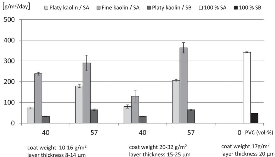
**Figure 3.** Normalized (15  $\mu\text{m}$  thickness) WVTR at 23°C and 85% relative humidity (RH) for kaolin with a shape factor of 30 (Fine kaolin) and 100 (Platy kaolin) combined with different amounts of SA and SB latex [35].
