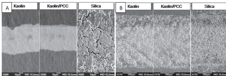
**Figure 8.** SEM images of silver particle inks printed with inkjet (A) and flexography (B) (3 g/m<sup>2</sup> top-coating). Reproduced with permission. Copyright 2012, Elsevier [29].
