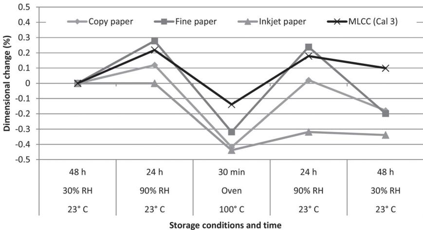
**Figure 11.** Dimensional change as function of humidity and temperature cycling for the different papers. Measurements are made after indicated time periods at each condition [37].
