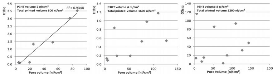
**Figure 10.** Surface resistivity as function of pore volume for 2 nl/cm<sup>2</sup> (left), 4 nl/cm<sup>2</sup> (middle) and 8 nl/cm<sup>2</sup> (right) total printed (roll-to-roll) semiconductor amounts. Reproduced with permission. Copyright 2012, Elsevier [29].
