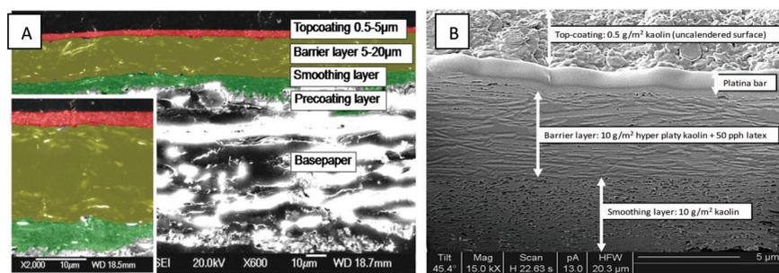
**Figure 1.** A: Cross-section scanning electron microscope (SEM) image showing the layer structure of the paper substrate: top-coating, barrier layer, smoothing layer, pre-coating and basepaper. Reproduced with permission. Copyright 2009, Elsevier [36]. B: Focused ion beam etched cross-section image. Reproduced with permission. Copyright 2012, Elsevier [29].
