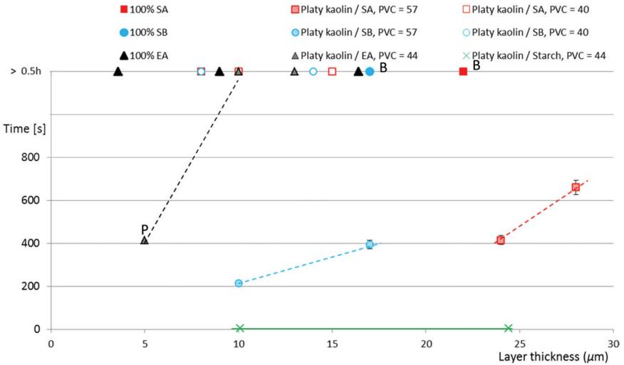
**Figure 7.** Barrier properties against 1 M hydrochloric acid. The figure shows the time in seconds for the liquid to penetrate the substrate. (B = Tendency for blocking, P = risk for pinholes). Penetration time measured with prism method presented in Figure 2B [50].
