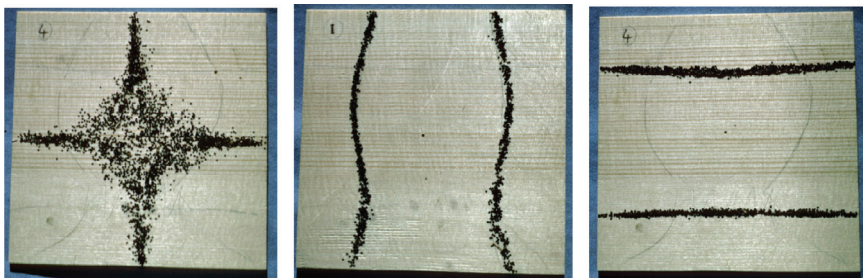
Figure 3. Chladni patterns illustrating three mode shapes of a thin wooden plate
