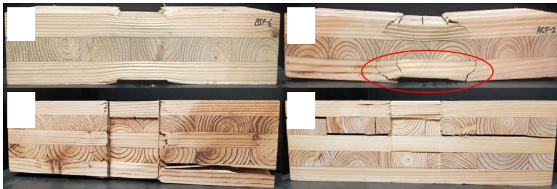
Fig. 4. Failure modes of the compression test specimens (Song 2018)
