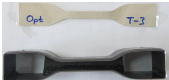
Fig. 1. Bio-hybrid film dog-bone sample for mechanical test and a cutting die for preparing the samples.
