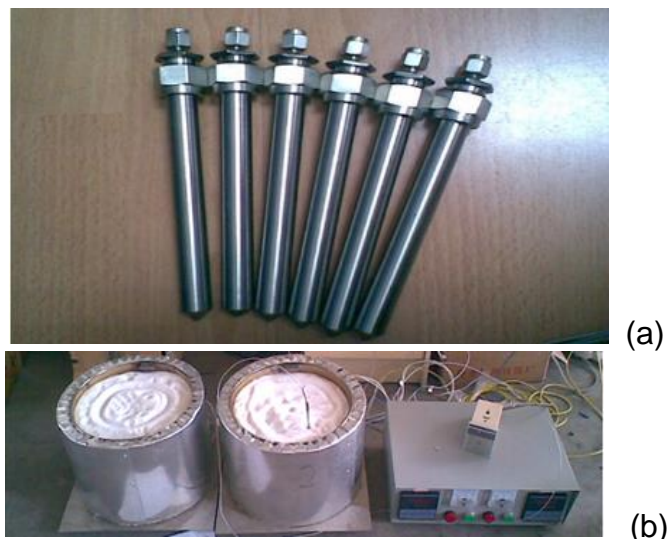
Fig. 1. (a) 15-mL tubular reactors and (b) the sand baths and the temperature controller
