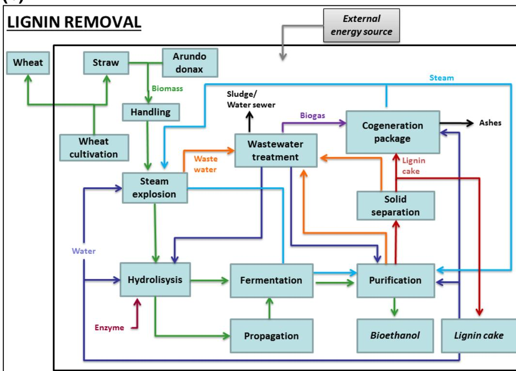
Fig. 1. System boundaries in bio-ethanol production. (a) Baseline scenario, (b) partial lignin removal scenario
