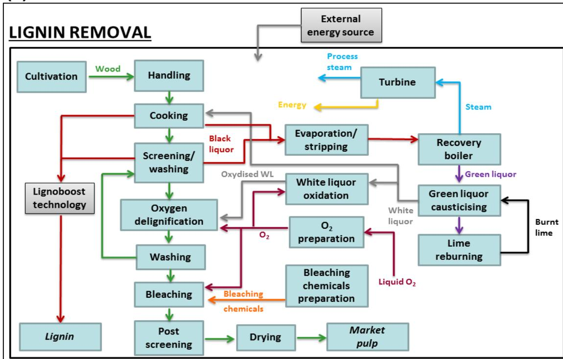
Fig. 2. System boundaries in softwood and hardwood pulp production (modified from: Suhr *et al.* 2015). (a) Baseline scenario, (b) partial lignin removal scenario
