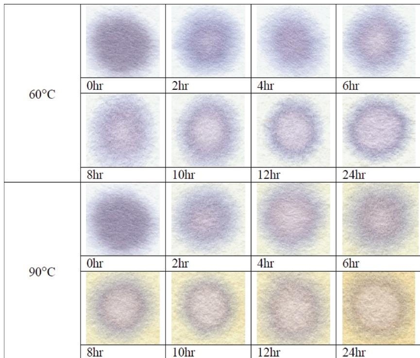
**Figure 3.** Aging of bioactive paper treated at 60°C and 90°C for various periods. The blue purple colour reveals the enzyme (ALP) – substrates (BCIP/NBT) reaction.
