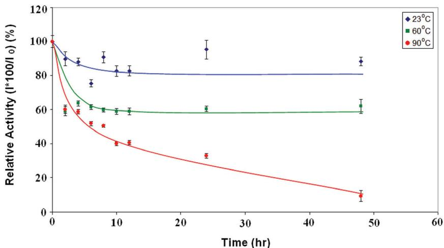
**Figure 4.** Effect of time and temperature on the activity of enzyme paper: ALP-paper; ( $I_0$  = grey value at 0hr and  $I$  = grey value at 't' hr).
