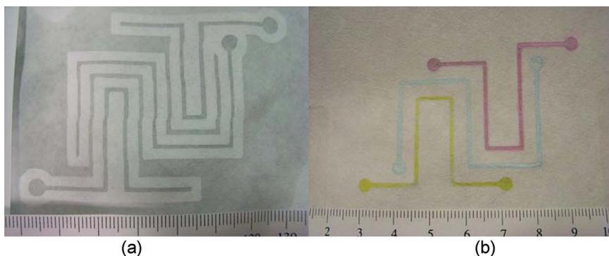
**Figure 6.** Paper printed microfluidic system as printed (a) and filled with three coloured liquids (b).
