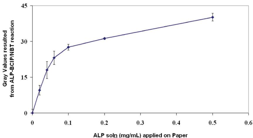
**Figure 2.** Calibration curve of gray values of the enzymatic products resulting from enzyme-substrate reaction on ALP enzymatic paper.
