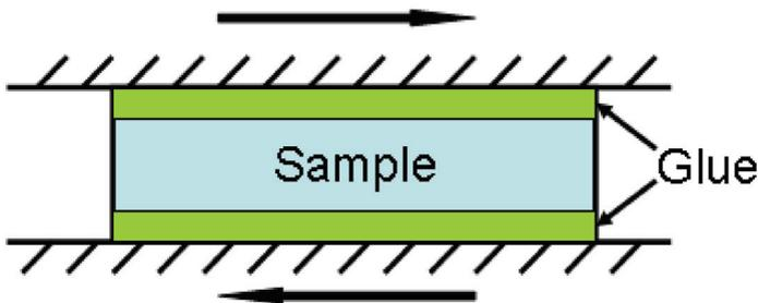
**Figure 1.** Schematic of rigid support shear methods; samples are glued.
