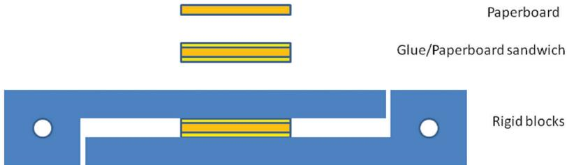
**Figure 4.** Schematic illustration of the manufacturing process of a rigid shear test (RST) specimen.
