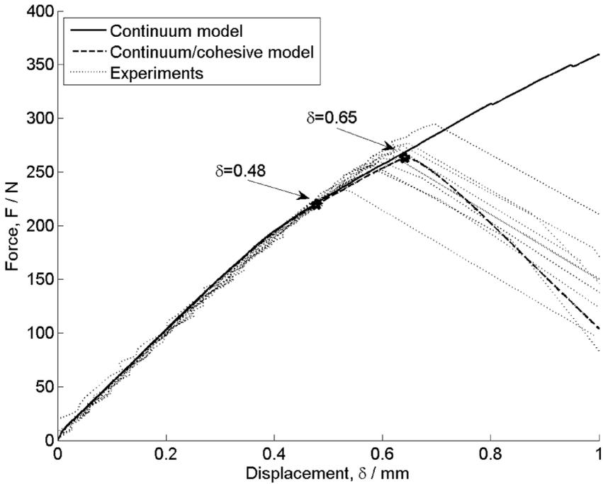
**Figure 9.** Force-displacement curves from the experimental and numerical tests of the NST specimen.
