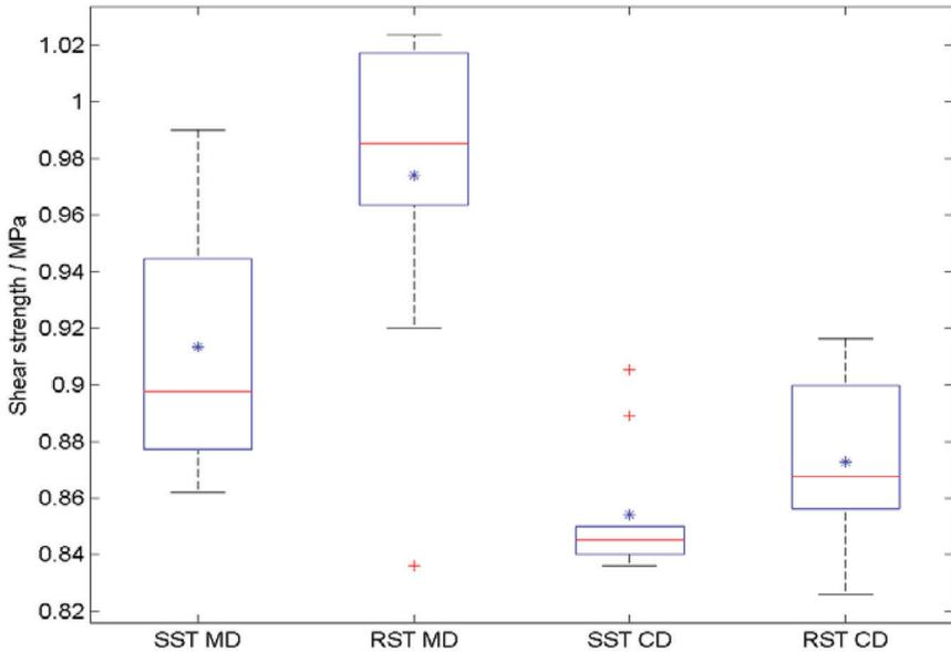
**Figure 5.** Measured shear strengths in MD and CD with SST and RST.
