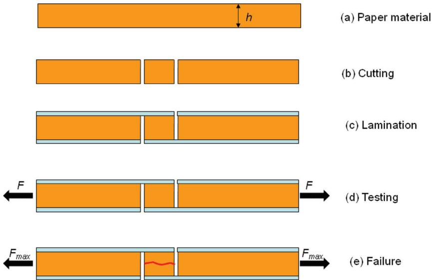
**Figure 3.** The manufacturing and testing procedure for the strip shear test (SST). (a) A paperboard with thickness  $h$  was the starting point, (b) two cuts were made, (c) the paperboard was laminated with plastic, (d) the sample was tested in a tensile testing machine, (e) failure occurred somewhere between the two cuts.
