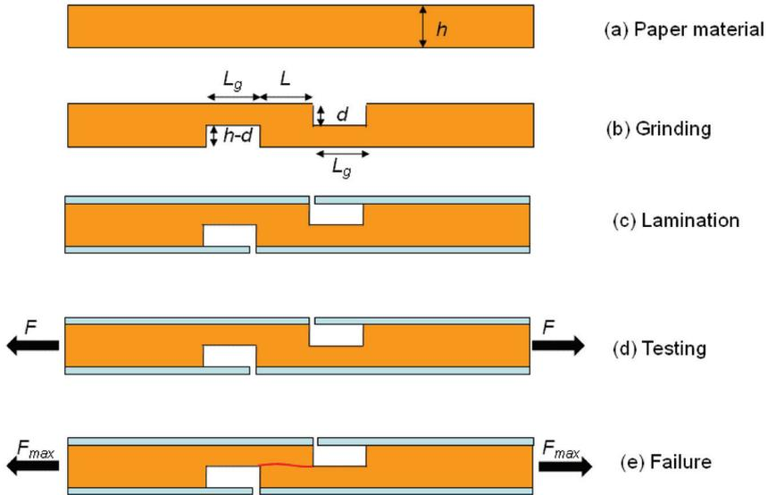
**Figure 2.** The manufacturing and testing procedure for the notched shear test (NST). (a) A paperboard with thickness  $h$  was the starting point, (b) two grooves were ground, (c) the paperboard was laminated with plastic, (d) the sample was tested in a tensile testing machine, (e) failure occurred between the two grooves.
