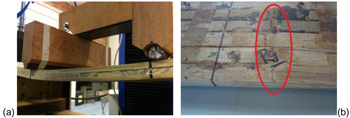
Fig. 9. Tested CLTB panels: (a) deflection, and (b) rupture in fibers (bottom part of panel).
