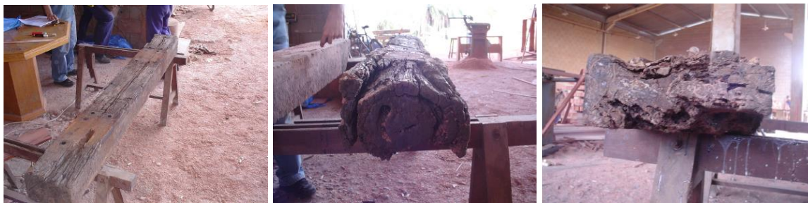
Fig. 1. Discharged sleepers classification. (a) half-way; (b) Scrap; (c) Firewood
