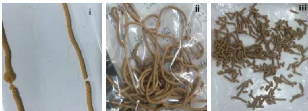
Fig. 2. Incense with different soy-based adhesive usage amounts (i) 44.4%, (ii) 31.8%, and (iii) 23.1%
