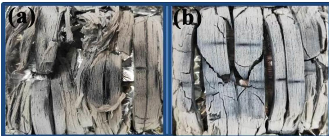
Fig. 11. Digital photographs of the residual charcoal: untreated bamboo (a), NLB (b)
