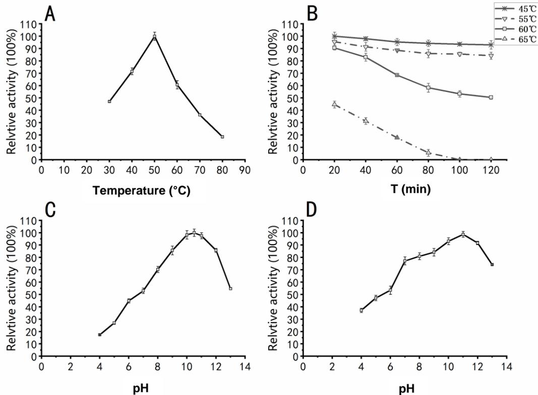
**Fig. 6.** Effects of temperature, pH, and NaCl on the activity and stability of the *aprD2*. (A) Effects of temperature on enzyme activity. (B) Stability of enzymes after incubation at 45 °C, 55 °C, 60 °C, and 65 °C for 0 to 120 min. (C) Effects of pH on enzyme activity. (D) pH stability of enzymes after incubation at pH 4-13 for 12 h. The experiment was repeated three times. Y-error bars show SEM of triplicate.
