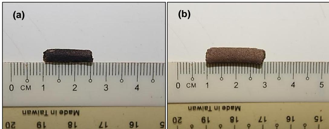
**Fig. 4.** Comparison of size between the OPEFB-SW (a) before water immersion and (b) after weeks of water immersion
