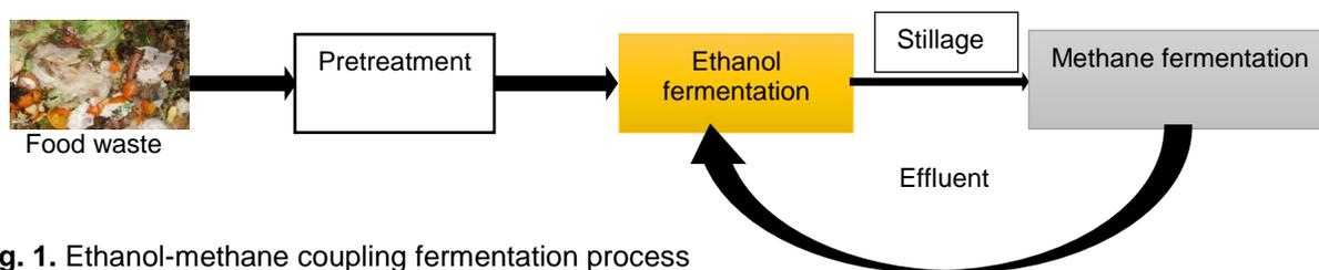
Fig. 1. Ethanol-methane coupling fermentation process
