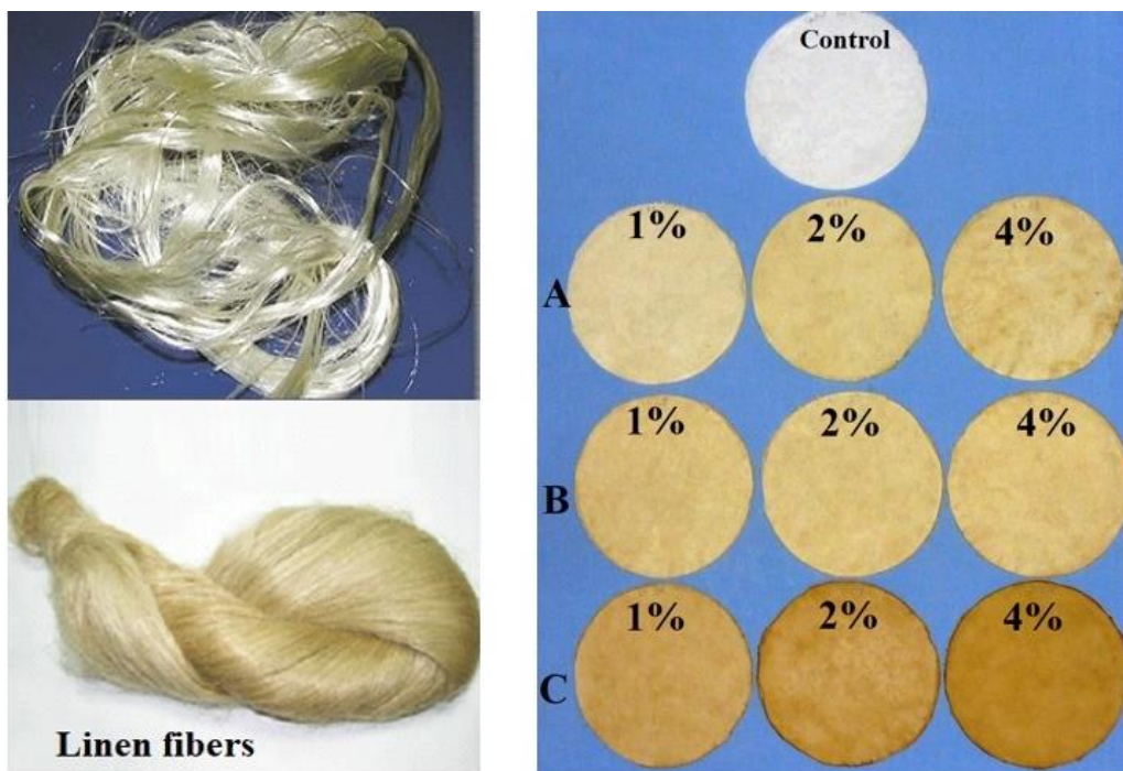
Fig. 1. Morphological photo for linen fibers and the manufactured laboratory papersheets from pulp with three additives.
