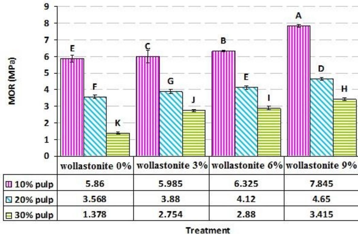
**Fig. 1.** Effect of varying levels of kraft pulp fiber and wollastonite on the MOR; letters on each column indicate Duncan's grouping at the 95% level of confidence
