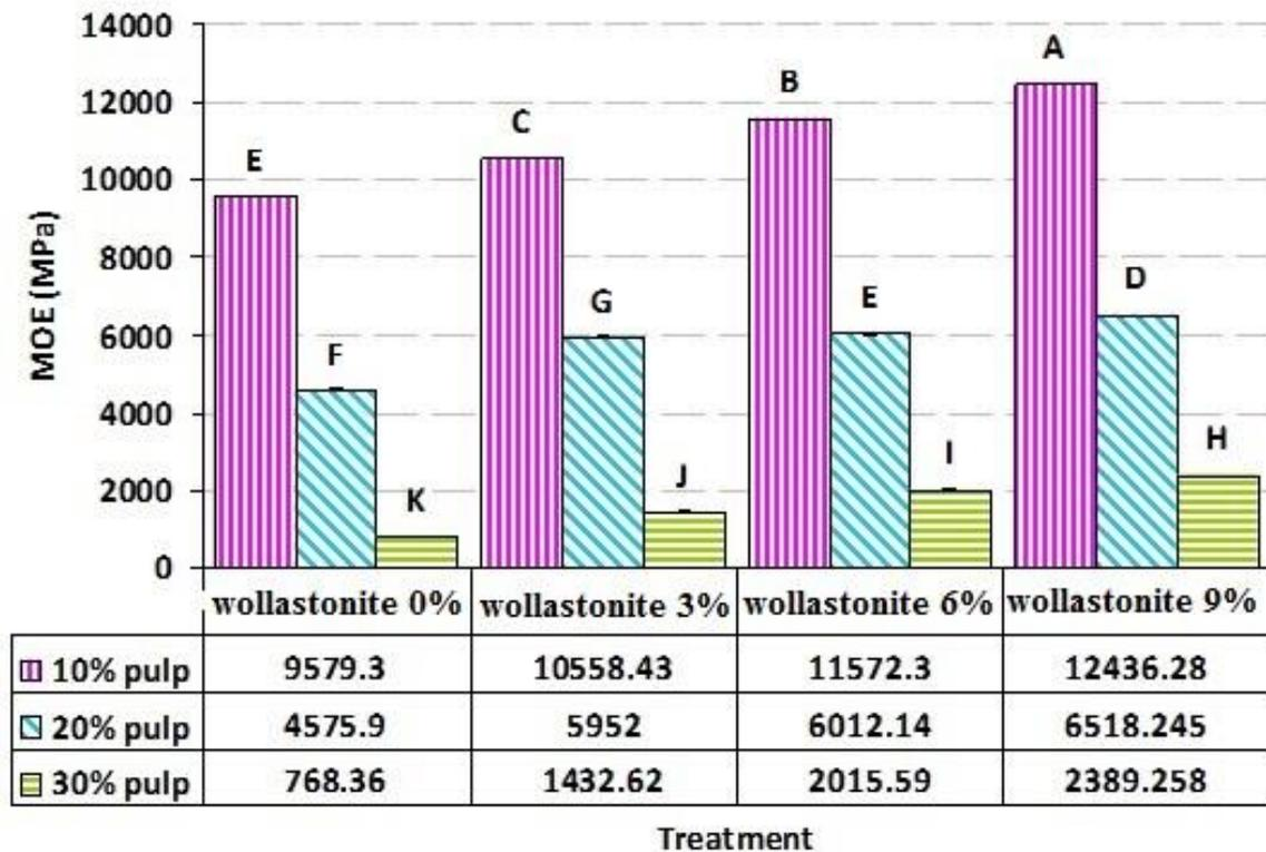
**Fig. 2.** Effect of varying levels of kraft pulp fiber and wollastonite on the MOE; letters on each column indicate Duncan's grouping at the 95% level of confidence
