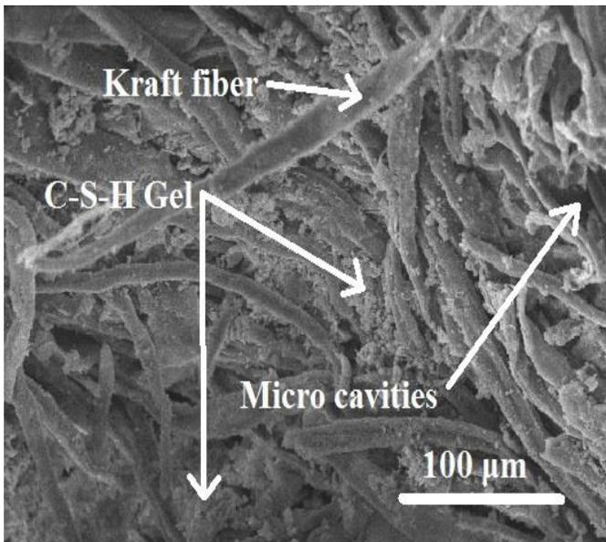
**Fig. 5c.** SEM image of fiber-cement composites with 6% wollastonite
