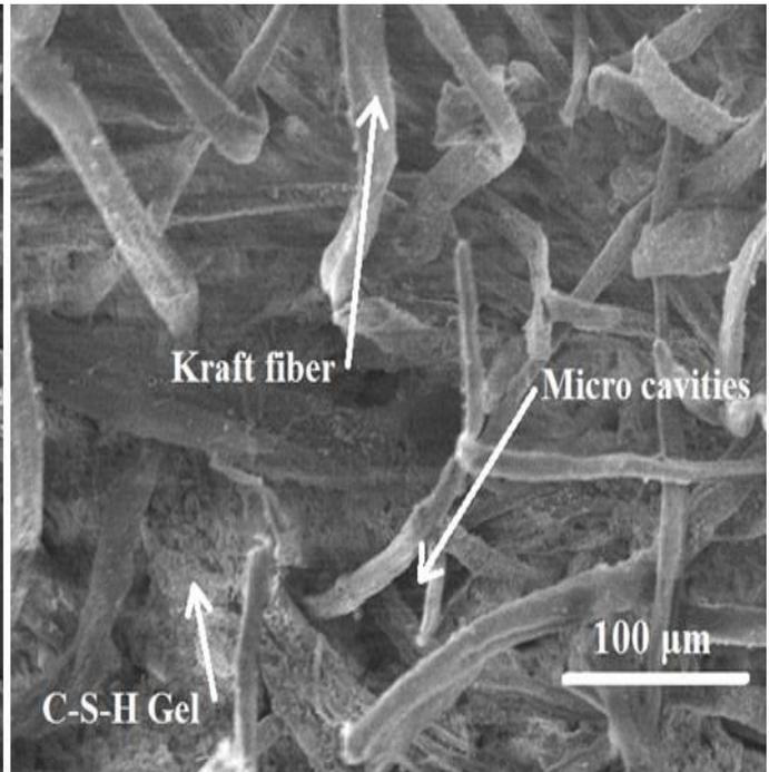
**Fig. 5b.** SEM image of fiber-cement composites with 3% wollastonite
