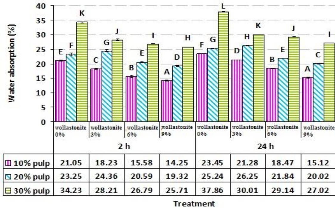
Fig. 3. Effect of varying levels of kraft pulp fiber and wollastonite on the water absorption (WA); letters on each column indicate Duncan's grouping at the 95% level of confidence
