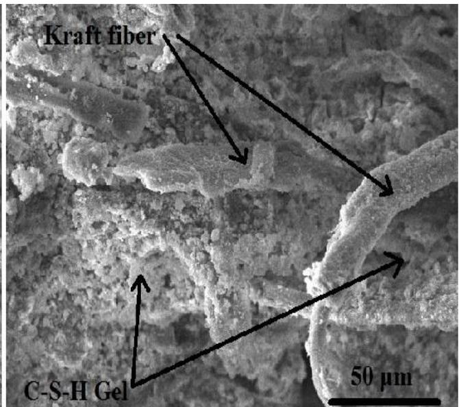
**Fig. 5d.** SEM image of fiber-cement composites with 9% wollastonite
