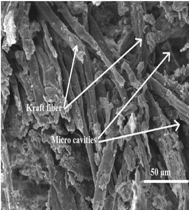
**Fig. 5a.** Weak structure of cement composites without wollastonite
