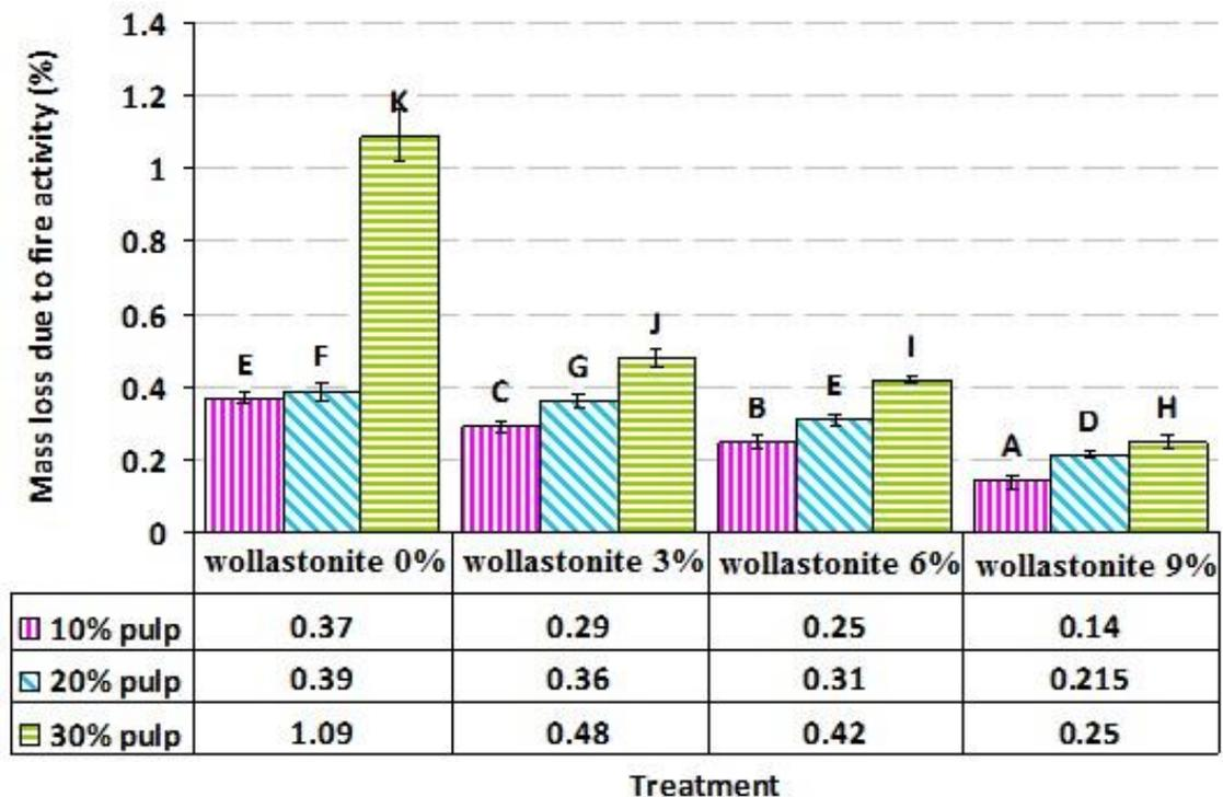
Fig. 4. Effect of varying levels of kraft pulp fiber and wollastonite on the mass loss (ML) due to fire exposing; letters on each column indicate Duncan's grouping at the 95% level of confidence
