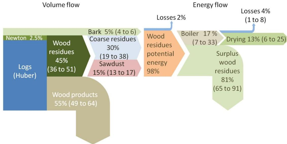
**Fig. 2.** Diagram of volume and energy flow of beech sawmill production (ranges of average data per group of logs are given in parentheses)
