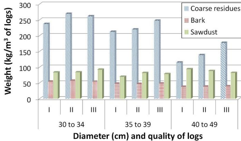
**Fig. 1.** Weight of wood residues per m<sup>3</sup> of logs with assumed MC (50% for coarse residues and bark, 30% for sawdust)
