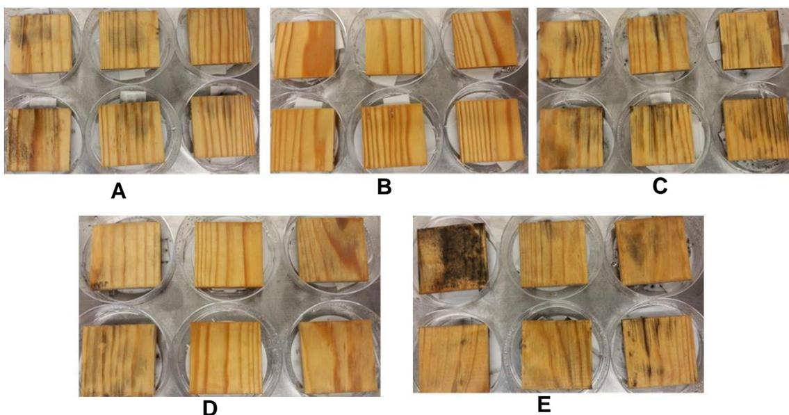
**Fig. 4.** Samples inoculated with *A. pullulans* after 8 weeks: (A) without silver nanoparticles, (B) with 0.1% IPBC + 1% propiconazole, (C) with 0.03% silver nanoparticles, (D) with 0.06% silver nanoparticles, and (E) with 0.09% silver nanoparticles
