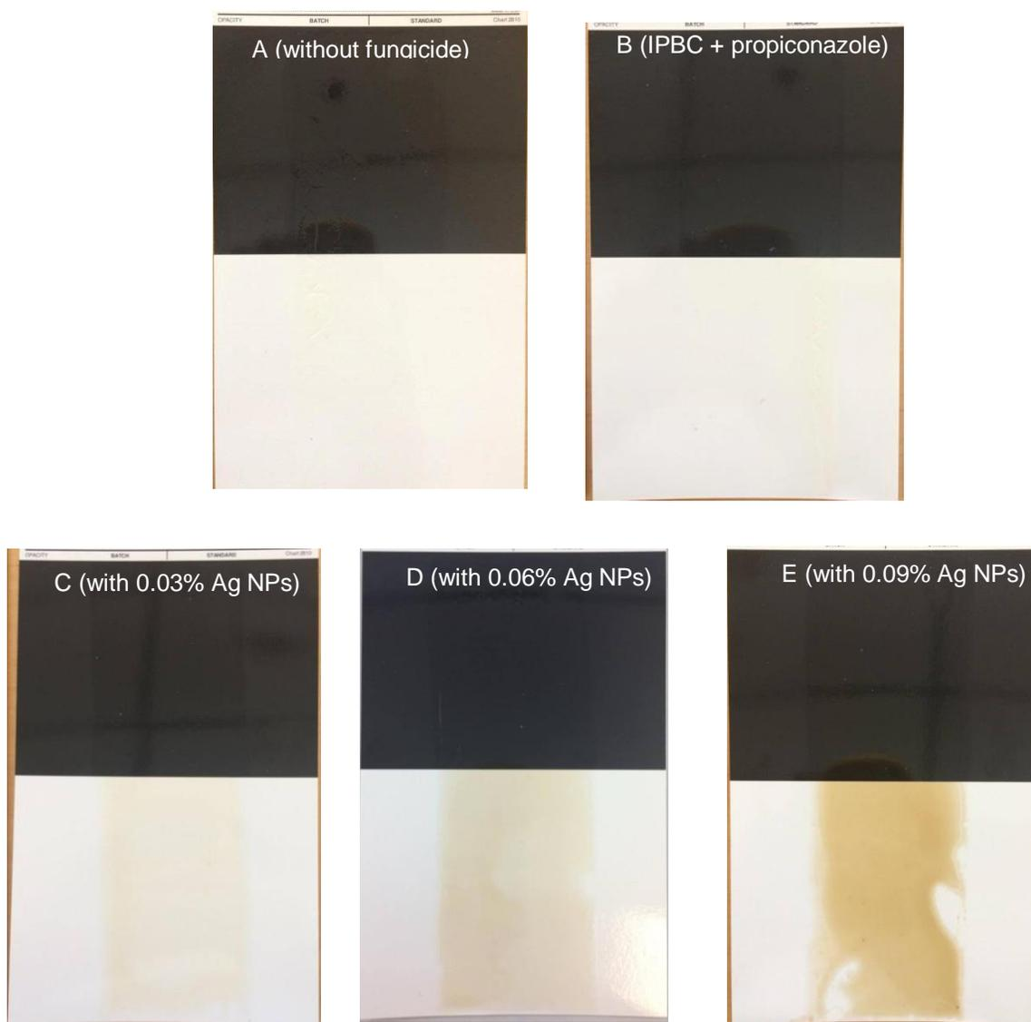
**Fig. 9.** Leneta contrast charts for the five coating formulations given in Table 1
