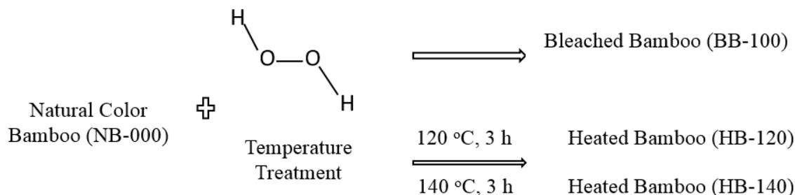
Fig. 1. Experimental framework for the bleaching and heat treatment process
