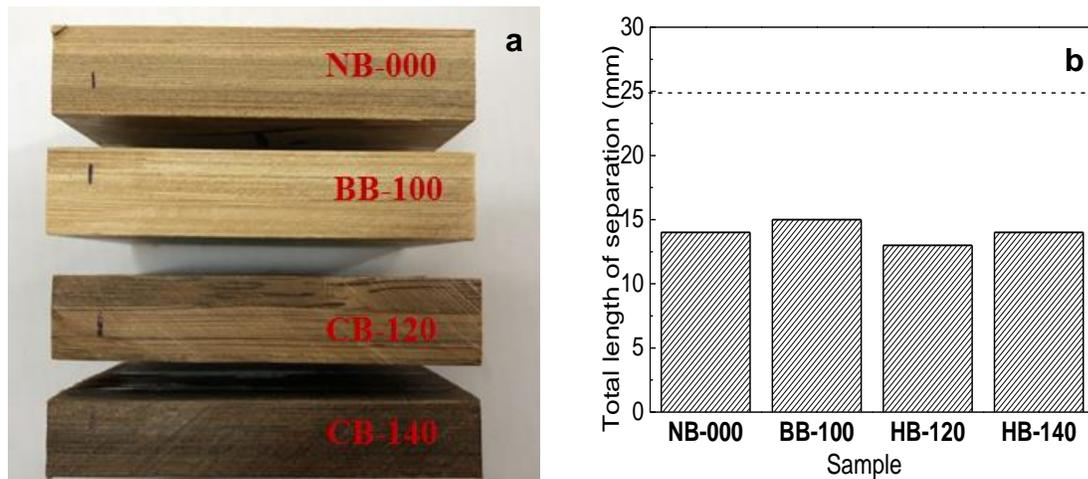
**Fig. 5.** (a) Visual examination of the bamboo samples and (b) the total length of separation for the sliver laminated bamboo adhesive film
