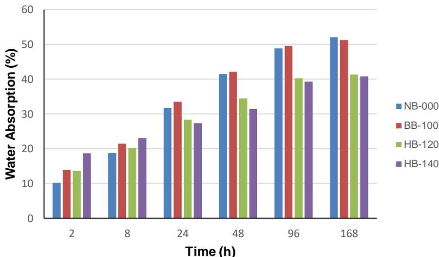
**Fig. 3.** The water absorption after the bleaching and heat treatment
