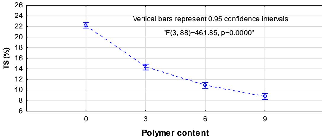
**Fig. 5.** The effect of the thermoplastic polymer on board swelling following 24 h immersion in water
