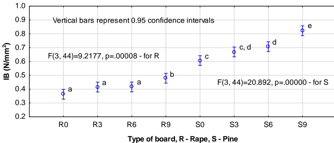
**Fig. 3.** Internal bonding strength of the board for rape straw boards and for pine chipboards enriched with PE (Letters mark uniform groups determined with the Tukey HSD test)
