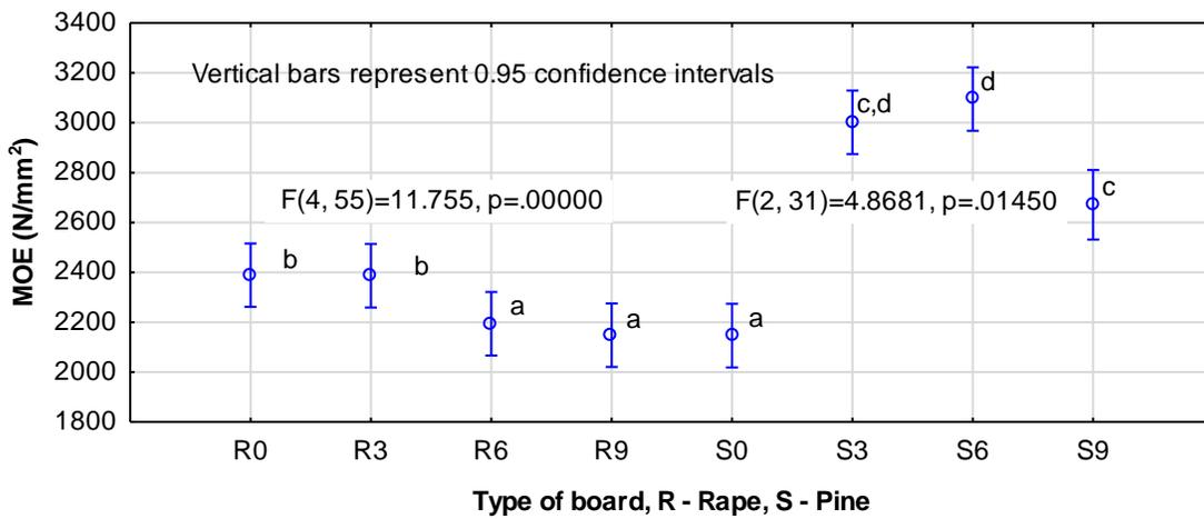
**Fig. 2.** Modulus of elasticity for pine chip boards and for rape straw boards enriched with PE (Letters mark uniform groups determined with the Tukey HSD test)
