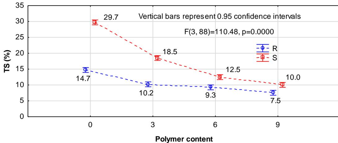
**Fig. 6.** An evaluation of interactions between the type of board material and the quantity of thermoplastic polymer, and swelling following 24 h immersion in water
