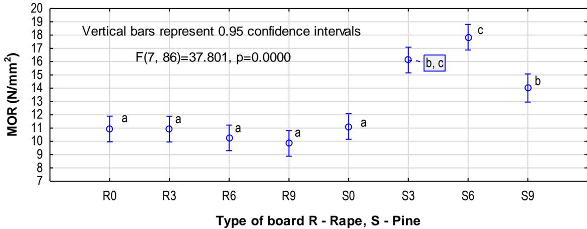
**Fig. 1.** Modulus of rupture for pine chip boards and for rape straw boards enriched with PE (Letters mark uniform groups determined with the Tukey HSD test)
