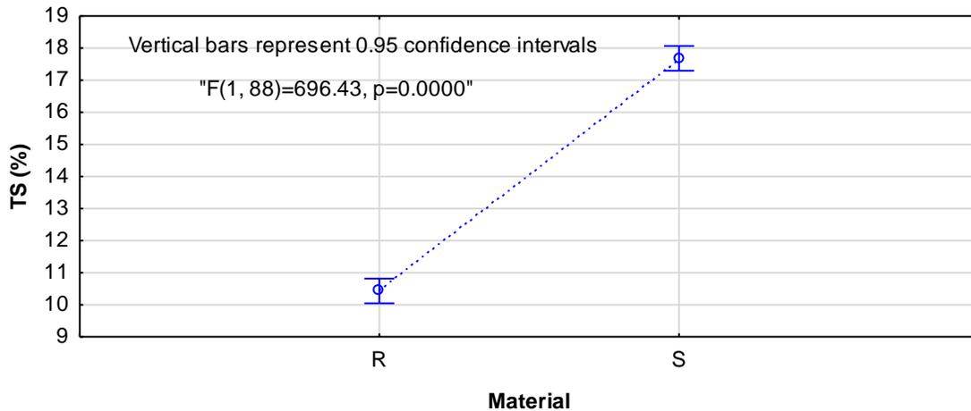
**Fig. 4.** An effect of the material on board swelling following 24 h immersion in water
