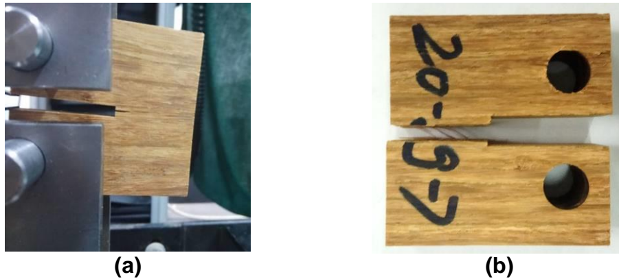
Fig. 6. Fracture of the specimen: (a) crack of the specimen and (b) fiber bridging
