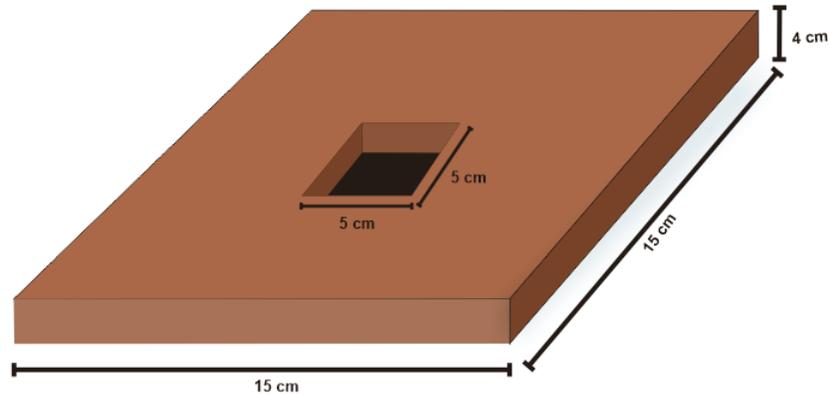
**Fig. 4.** Custom holder for small wood block sample testing
