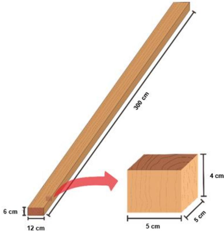
**Fig. 1.** Illustration of small wood block samples cut from *Shorea* spp. lumber
