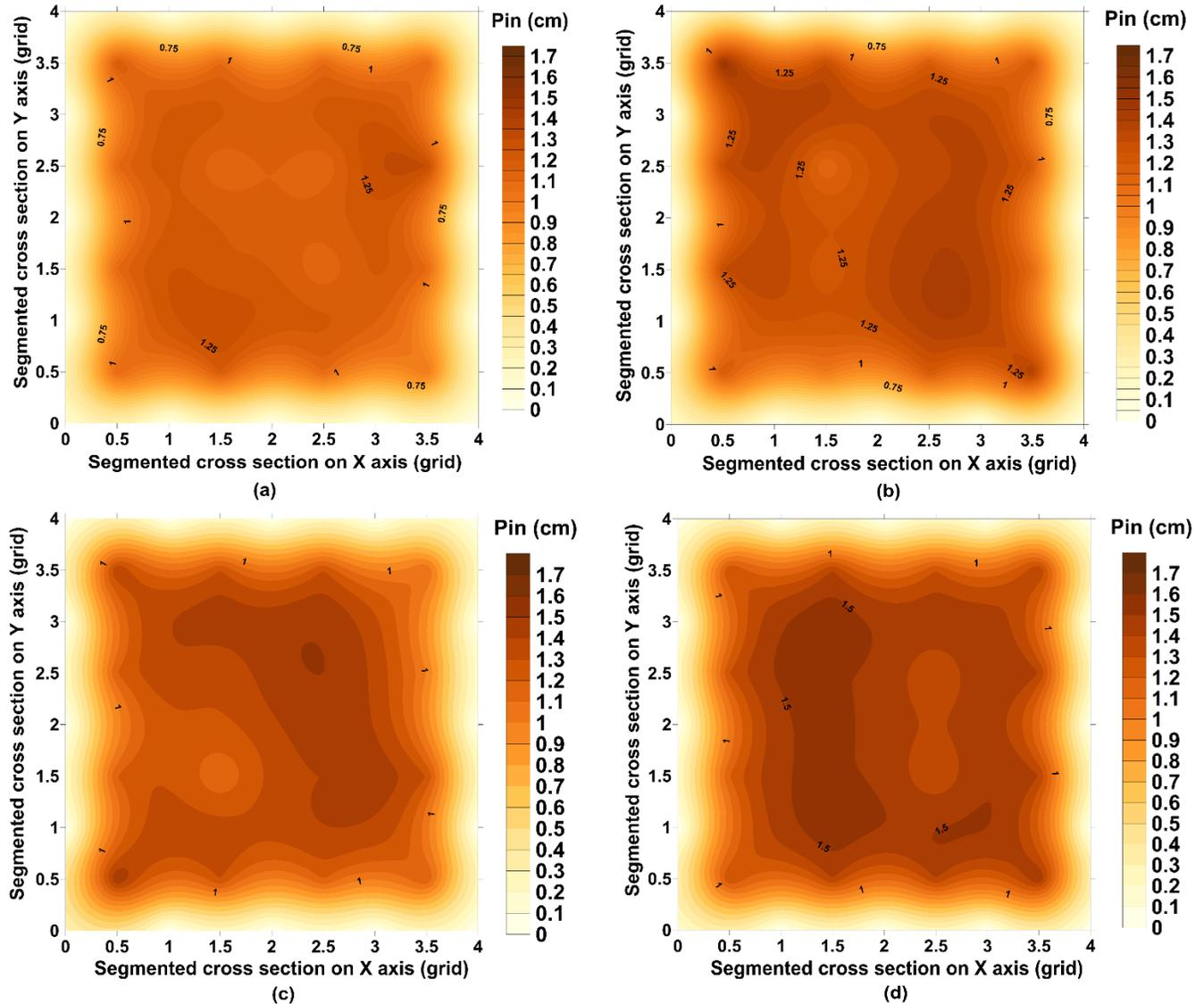
**Fig. 9.** Distribution of pin penetration depths of samples taken from: unexposed (a), 3 weeks exposed (b), 6 weeks exposed (c), and 9 weeks exposed (d), the small wood block sample group
