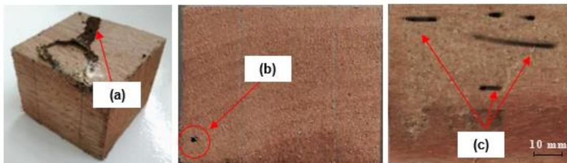
**Fig. 6.** Termite tunnel (a), entrance hole (b), and gallery pattern (c) on the infested small wood block samples
