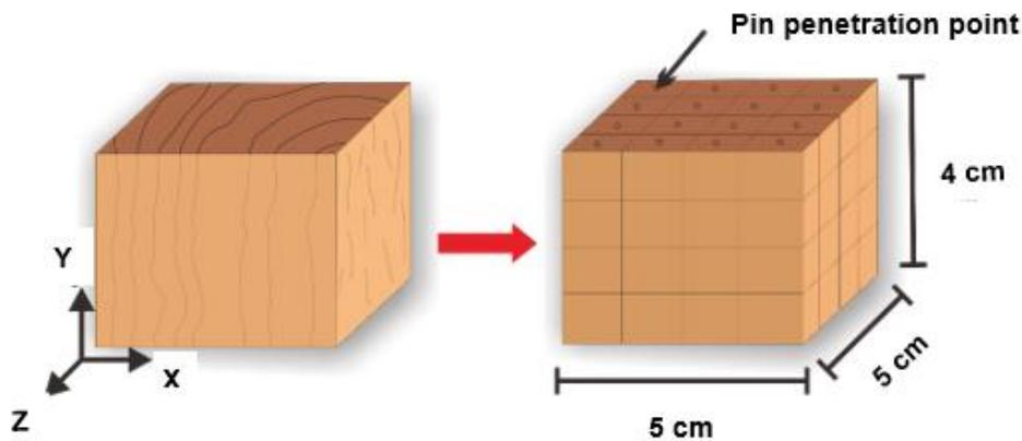
**Fig. 3.** Small wood block sample preparation for pin penetration test
