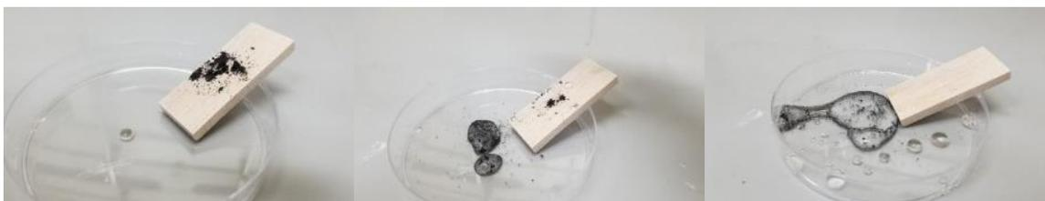
**Fig. 3.** Snapshots of the self-cleaning process on the superhydrophobic wood surfaces
