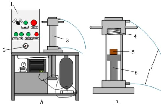
**Fig. S1.** The lab-scale dewatering system
