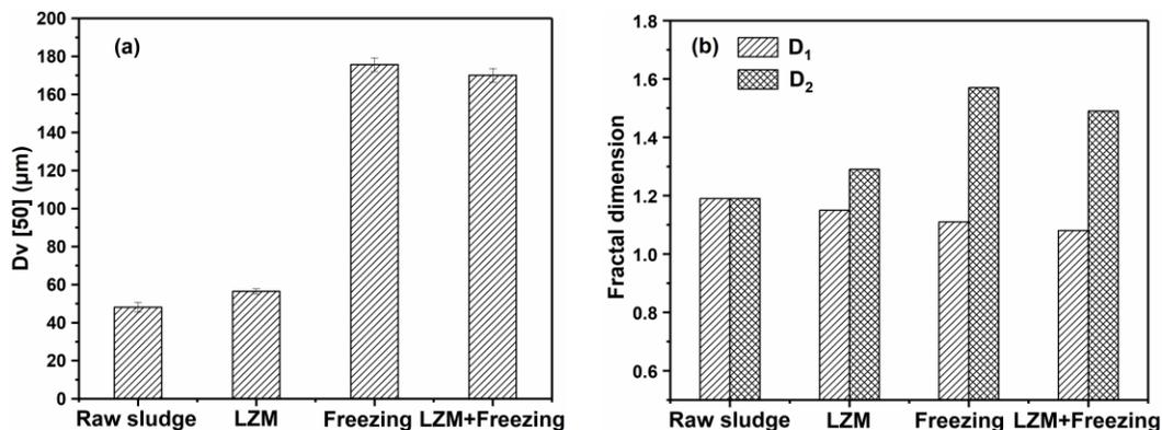
**Fig. 3.** Sludge particle size distribution (a)  $D_v [50]$ ; (b) Fractal dimension
