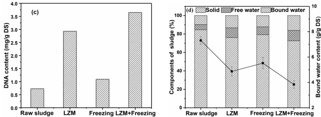
**Fig. 2.** Effects of various conditioning methods on EPS components, bound water and DNA content: (a) Protein; (b) Polysaccharide; (c) DNA and (d) Bound water
