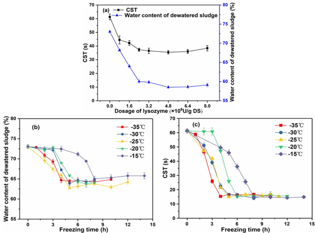
**Fig. S2.** Effects of separate conditioning on sludge dewatering performance (a) LZM; (b) and (c) Freeze-thaw
