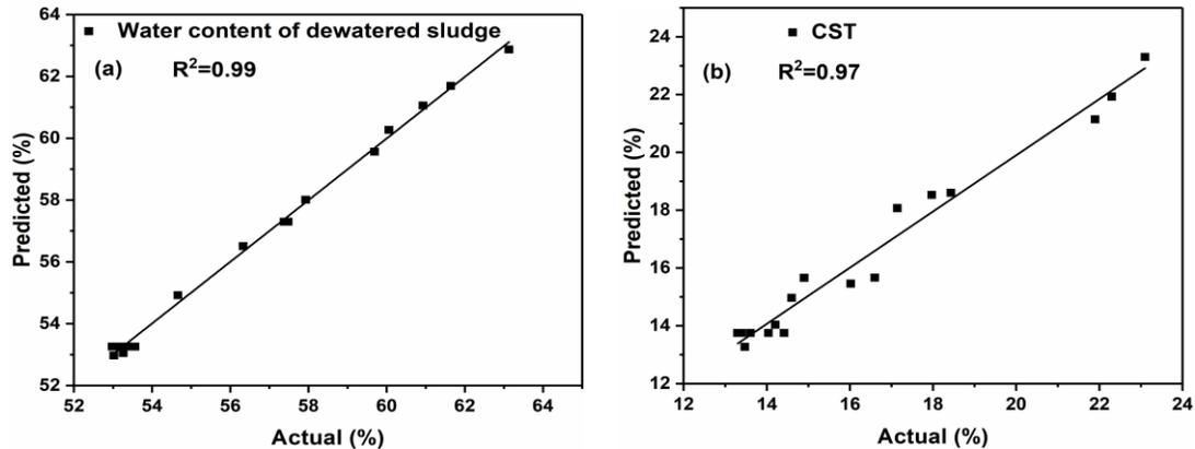
**Fig. 1.** Comparison of predicted and actual results: (a) Water content of the dewatered sludge and (b) CST
