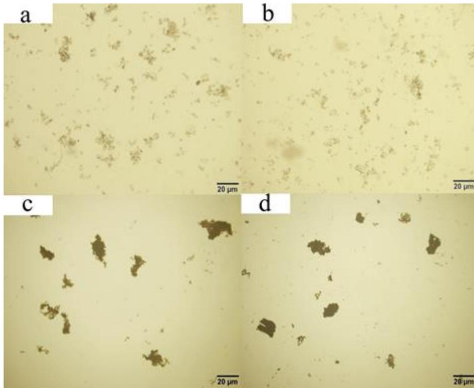
**Fig. S3.** Micrographs of sludge treated under various conditions (a) Raw sludge; (b) LZM; (c) Freezing; (d) LZM + freezing
