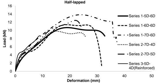
Fig. 8. Typical load-deformation curves of the half-lapped connection for the tension test
