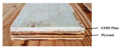
Fig. 1. Shape of reinforced plywood with GFRP plate
