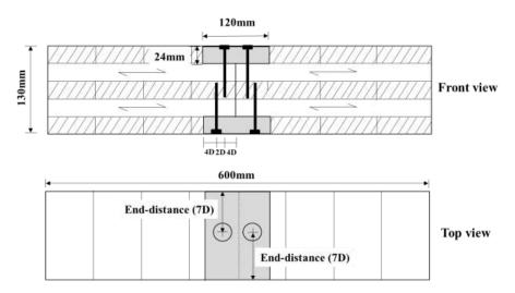
Fig. 5. Schematic diagrams of the double-spline connection specimen
