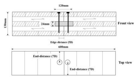
Fig. 4. Schematic diagrams of the internal spline connection specimen
