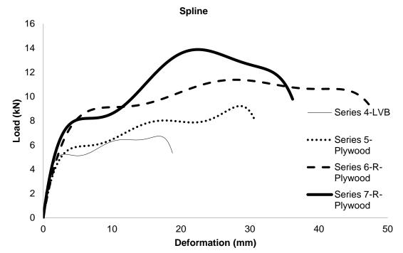
Fig. 9. Typical load-deformation curves of the spline connection for the tension test
