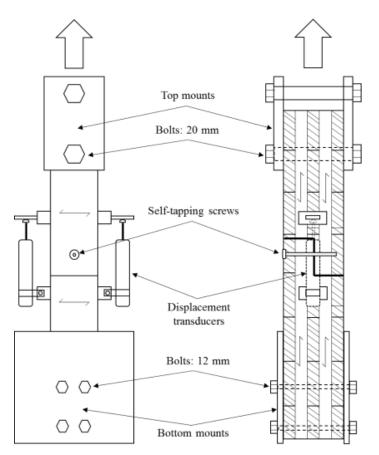
Fig. 7. Schematic diagram of the tension test on the edge connections between the CLT panels
