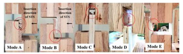
Fig. 10. Failure modes of the edge connections between the CLT panels
