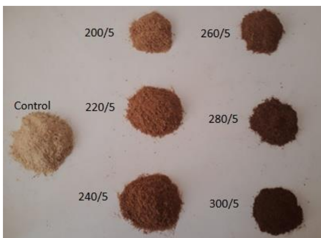
Fig. 2. Spruce sawdust samples used for 5 min torrefaction and temperature of 200 °C to 300 °C
