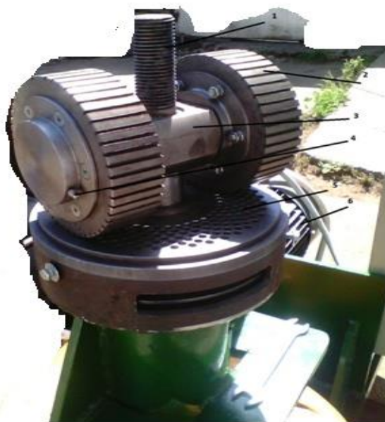
Fig. 3. Mechanical press for pelletisation (Group matrix –roles): 1-main screw; 2-roll; 3-roll support; 4-lubricat; 5-matrix; 6-motor
