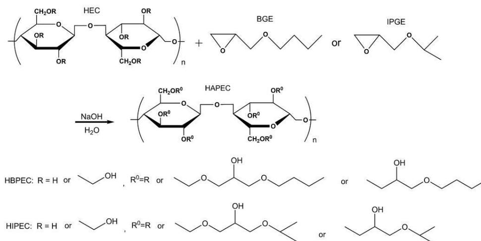
Fig. 1. Synthetic pathway of HBPEC and HIPEC
