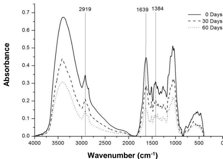
Fig. 3. The FTIR spectra of the composting samples on day 0, 30, and 60
