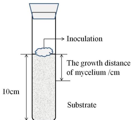
Fig. 1. Schematic diagram of the test-tube cultivation apparatus for the edible fungi
