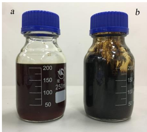
Fig. 5. Light (a) and heavy (b) bio-oil from birch wood pyrolysis
