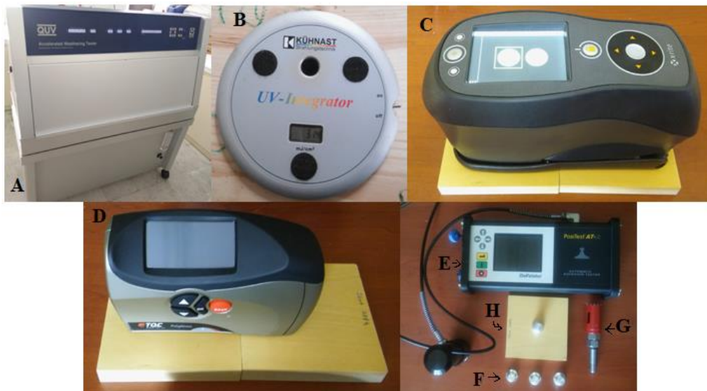
Fig. 1. (A) QUV weathering tester, (B) UV integrator, (C) X Rite Ci62 Series Portable, (D) Novo-Gloss Trio gloss meter, (E) PosiTest AT-A (automatic) pull-off adhesion tester, (F) dolly, (G) cutting tool, and (H) test sample
