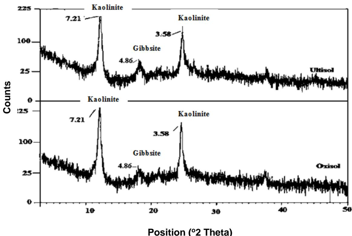
Fig. 1. X-ray diffractograms of the clay fraction of the soils under study
