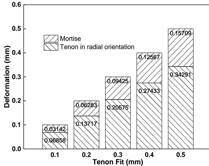
Fig. 7. Deformations of the mortise and tenon with a radial grain orientation and different tenon fits
