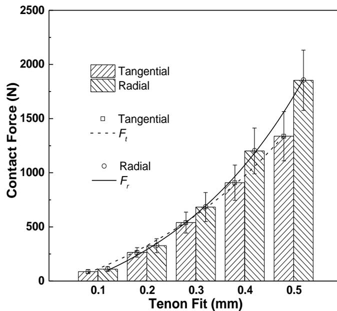
**Fig. 4.** Contact forces between the mortises and tenons with different tenon fits and grain orientations
