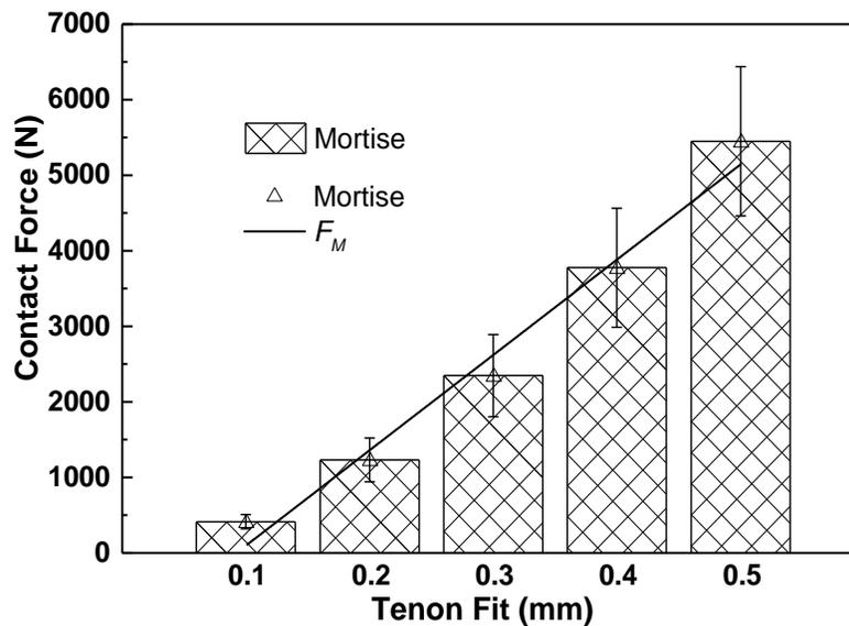
**Fig. 6.** Contact forces between the mortises and tenons with a steel-made tenon and different tenon fits
