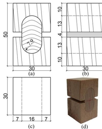
**Fig. 2.** Dimensions (mm) of the specimen: (a) front view, (b) left view, and (c) top view; and (d) photo of the specimen
