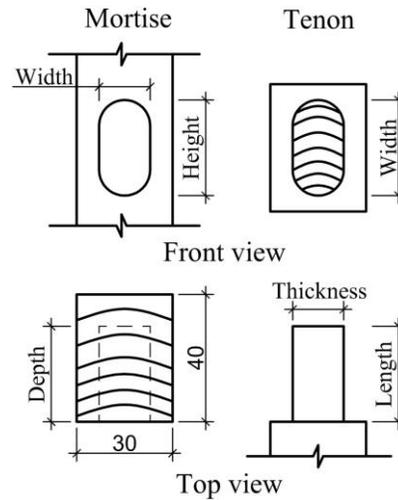
**Fig. 1.** Definition of tenon fit between mortise and tenon
