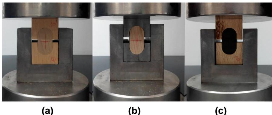
**Fig. 3.** Setup for measuring the (a) contact forces of the mortises and tenons, (b) stiffness of the tenon, and (c) stiffness of the mortise
