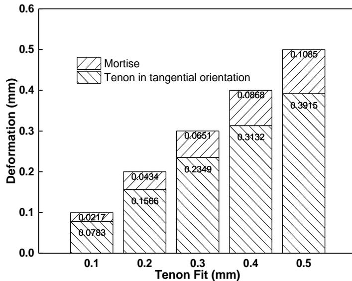
Fig. 8. Deformations of the mortise and tenon with a tangential grain orientation and different tenon fits
