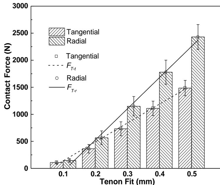
**Fig. 5.** Contact forces between the mortises and tenons with a steel-made mortise in different tenon fits and grain orientations
