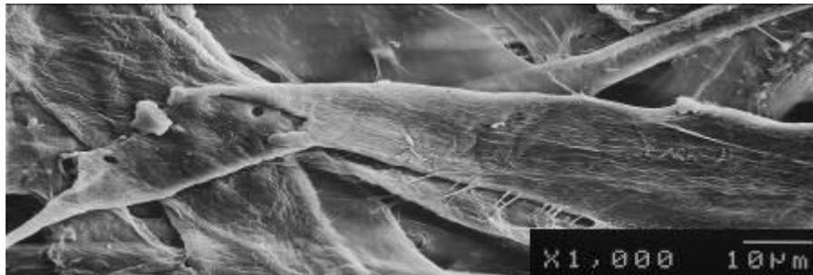
Fig. 10. The paper surface with 4% NFC addition
