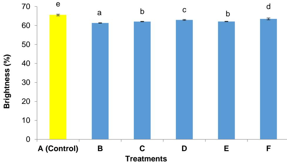
**Fig. 6.** Effect of NFC on brightness (B= 0% NFC, C= 2% NFC, D= 4% NFC, E= 6% NFC, F= 8% NFC)
