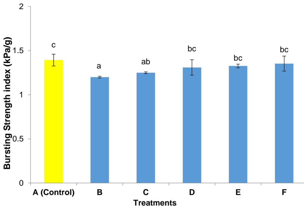
**Fig. 5.** Effect of NFC on the bursting strength index (B= 0% NFC, C= 2% NFC, D= 4% NFC, E= 6% NFC, F= 8% NFC)
