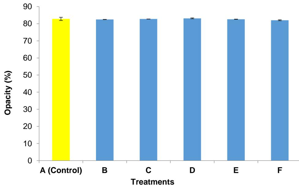
**Fig. 7.** Effect of NFC on opacity (B= 0% NFC, C= 2% NFC, D= 4% NFC, E= 6% NFC, F= 8% NFC)
