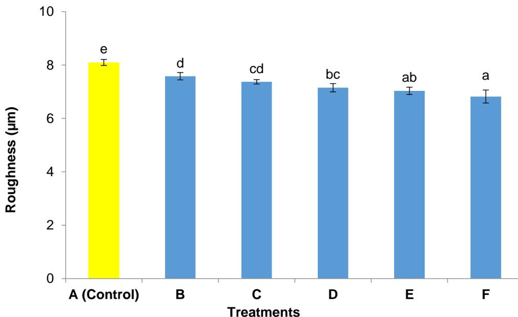
**Fig. 1.** The effect of NFC on the roughness (B= 0% NFC, C= 2% NFC, D= 4% NFC, E= 6% NFC, F= 8% NFC)
