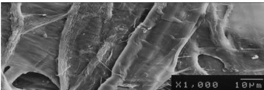
Fig. 11. The paper surface with 8% NFC addition
