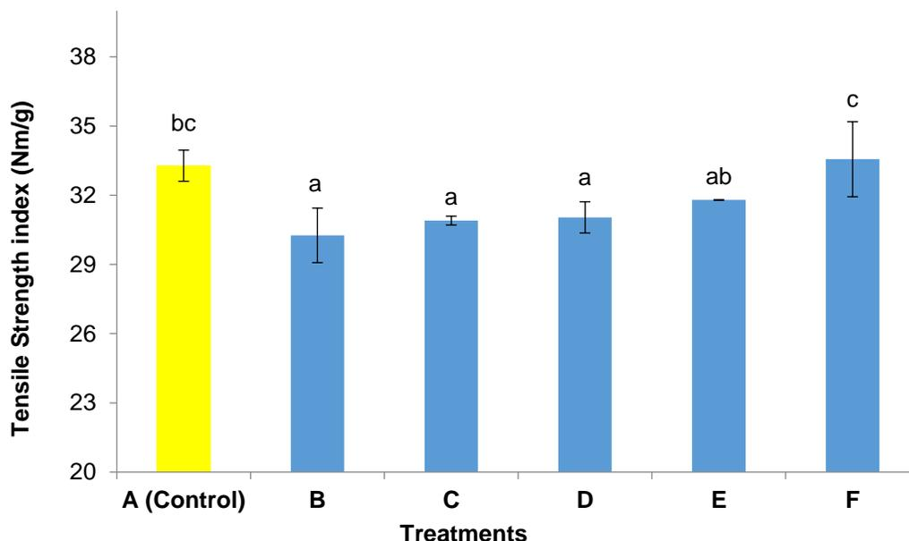
**Fig. 3.** The effect of NFC on the tensile strength index (B= 0% NFC, C= 2% NFC, D= 4% NFC, E= 6% NFC, F= 8% NFC)
