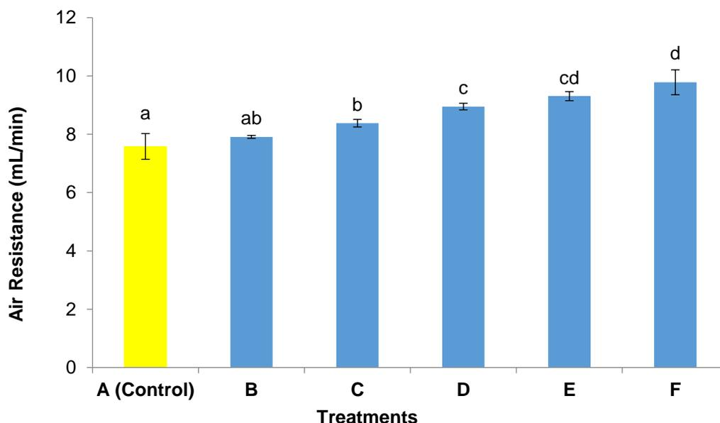
**Fig. 2.** The effect of NFC on the air resistance (B= 0% NFC, C= 2% NFC, D= 4% NFC, E= 6% NFC, F= 8% NFC)
