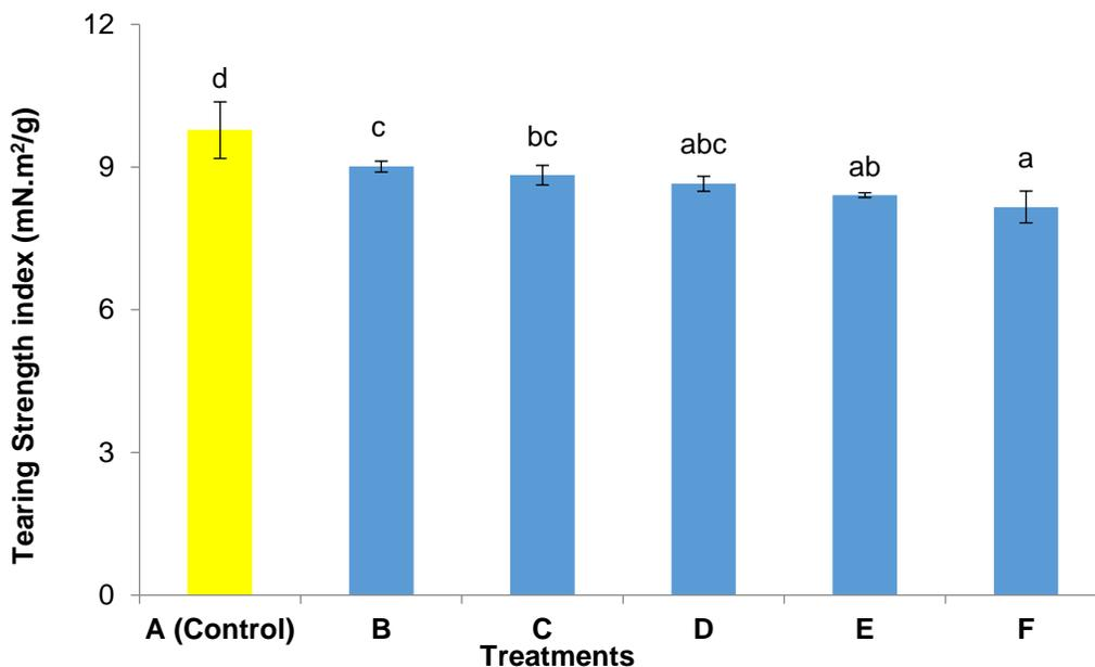
**Fig. 4.** The effect of NFC on the tear strength index (B= 0% NFC, C= 2% NFC, D= 4% NFC, E= 6% NFC, F= 8% NFC)
