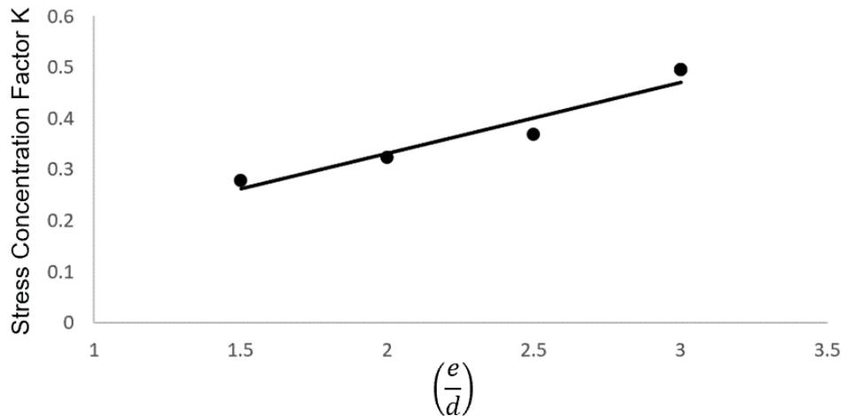
**Fig. 10.** Mean values of stress concentration factor,  $K$ , were plotted as a function of end-or edge-distance to bolt-diameter ratio,  $(e/d)$ , for single-shear unconstrained wood-plastic composite-to-metal single-bolt connections failed in end tear-out and net cross-section modes
