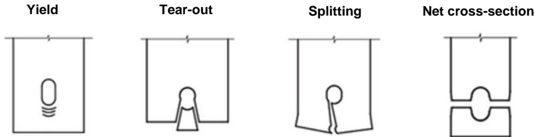
**Fig. 1.** Four types of failure modes commonly seen in a single-shear metal-to-wood or wood-based composite single-bolt connection
