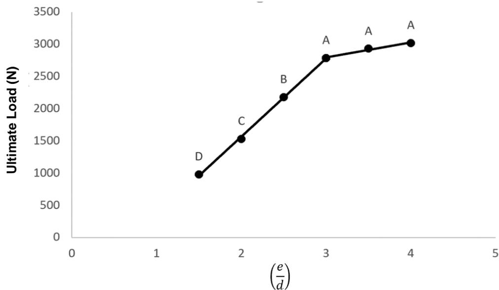
**Fig. 9.** Mean ultimate lateral loads of SUWSCs evaluated in this study as a function of  $(\frac{e}{d})$
