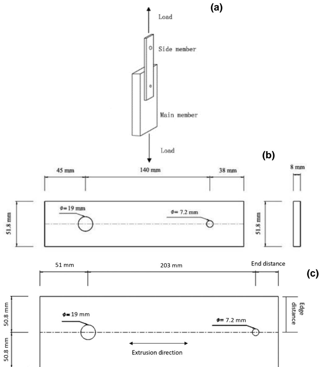
**Fig. 2.** General configurations of (a) a single-shear unconstrained WPC-to-metal single-bolt connection, (b) detailed dimensions of a metal plate side member, and (c) WPC main member parallel its extrusion direction
