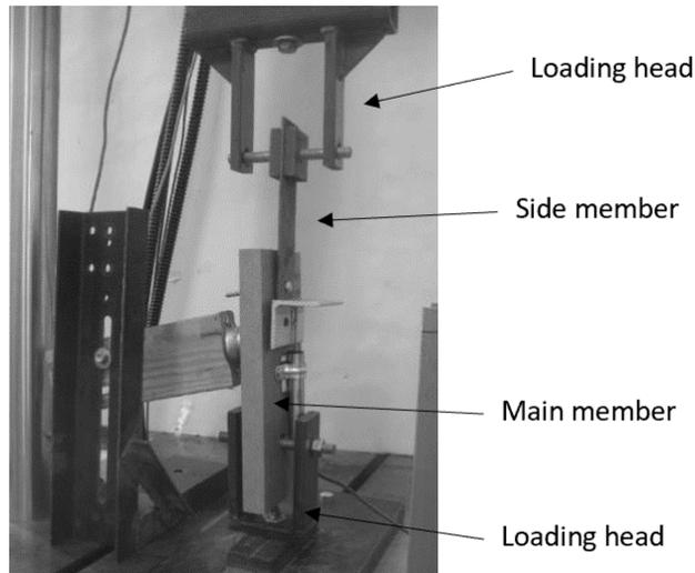
**Fig. 7.** Test setups for evaluating ultimate lateral resistance loads of unconstrained single-shear single-bolt connections in wood-plastic composite lumber parallel to its extrusion direction
