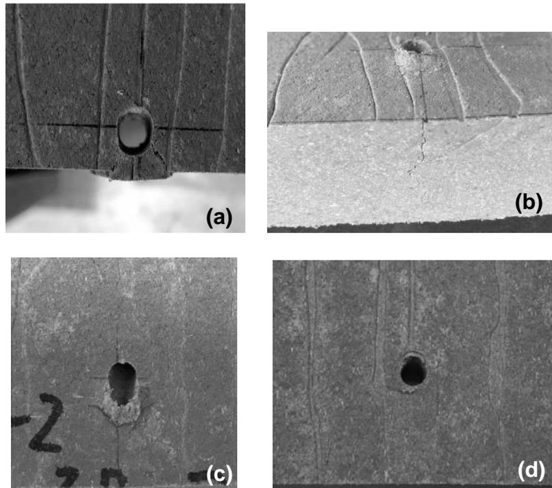
**Fig. 8.** Typical failure modes observed in evaluating the ultimate lateral load of single-shear unconstrained WPC-to-metal single-bolt connections when subjected to static lateral loading parallel to the WPC extrusion direction: end tear-out (a); end splitting (b); material compressively fractured at the end closest to (c) and away from (d) the metal plate
