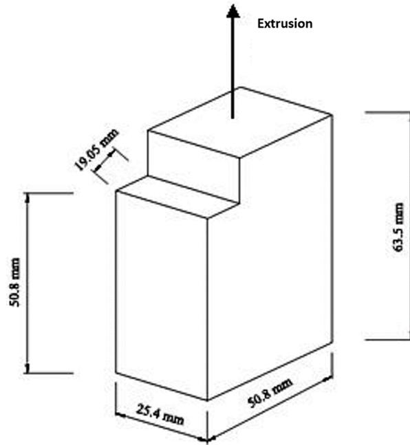
**Fig. 3.** General configuration of specimens used in this study for testing shear strengths of wood-plastic composite lumber parallel to its extrusion direction
