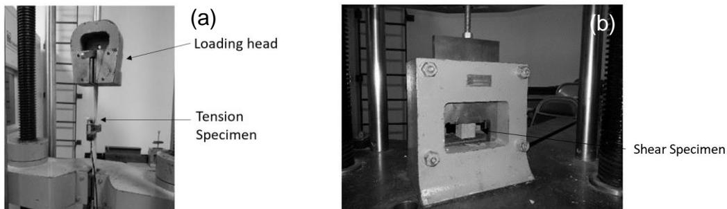
**Fig. 6.** Test setups for evaluating tensile (a) and shear (b) strengths of WPC lumber used in this study
