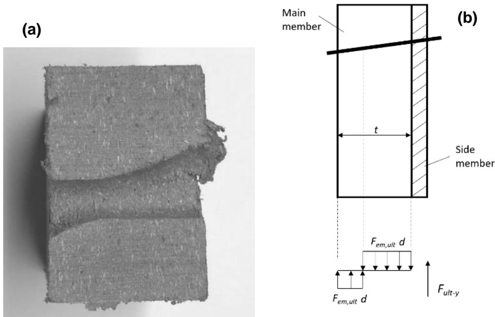
**Fig. 11.** The typical deformed shape (a), and the mechanical model of single-shear unconstrained wood-plastic composite-to-metal single-bolt connections subjected to static lateral loads parallel to the WPC extrusion direction (b)
