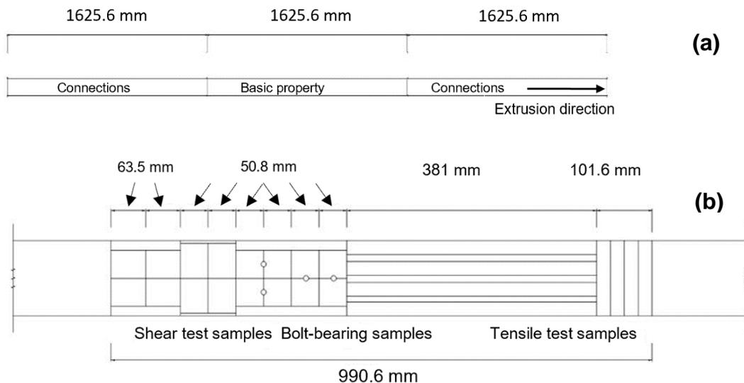
**Fig. 5.** Cutting patterns showing: (a) where WPC mechanical property and connection specimens were cut from full-size WPC lumber and (b) how WPC mechanical property specimens were cut
