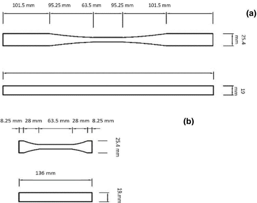
**Fig. 4.** General configurations of specimens used in this study for testing tensile strengths of wood-plastic composite lumber parallel (a) and perpendicular (b) to its extrusion direction
