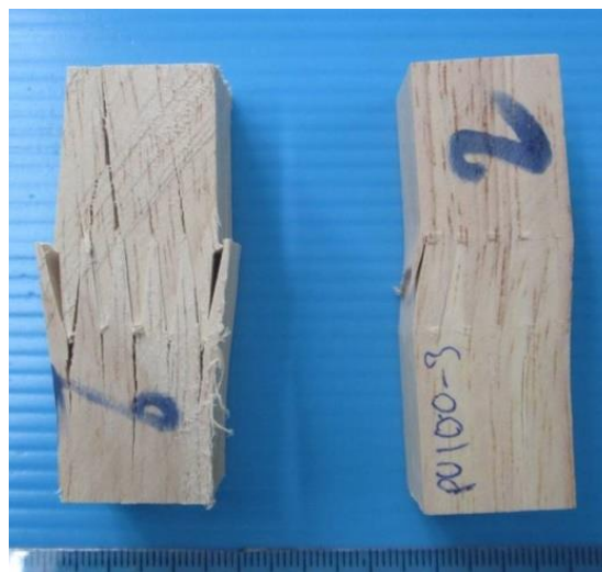
Fig. 3. Typical failure modes of finger jointed specimens after compression parallel to the grain test
